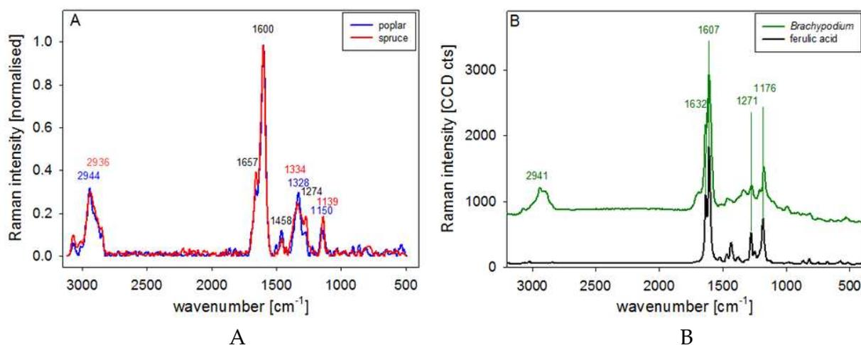
**Figure 4. A-B.** Raman spectra (532 nm excitation, 0.1-0.4 s integration time) acquired from the cell corner of wood (poplar and spruce, A) and *Brachypodium* (B), reflecting the different lignin structures in softwood, hardwood and grasses. Additionally a reference spectrum of ferulic acid is plotted (B, black line)
