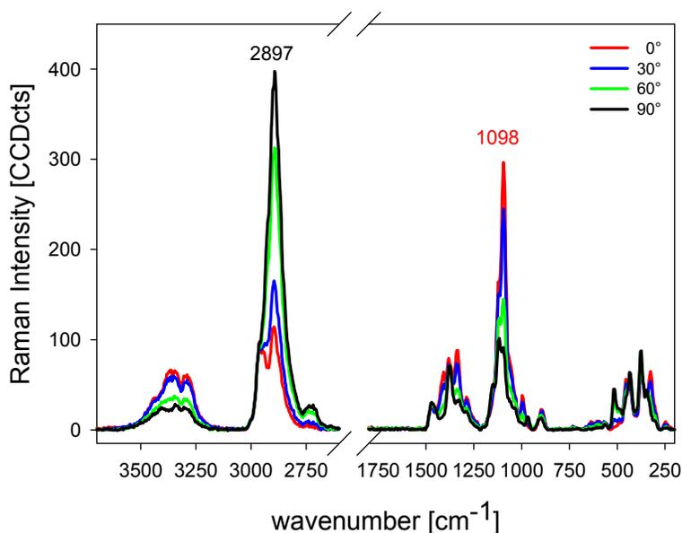
**Figure 2.** Raman spectra (532 nm excitation, 0.25 s integration time, 10 accumulations, baseline corrected) acquired from a Ramie fibre (>95% cellulose, high crystallinity, microfibrils aligned parallel to the fibre axis) with changing the polarization direction of the incident laser from  $0^\circ$  (parallel to the fibre axis and cellulose fibrils) to  $90^\circ$  (perpendicular to the fibre axis).
