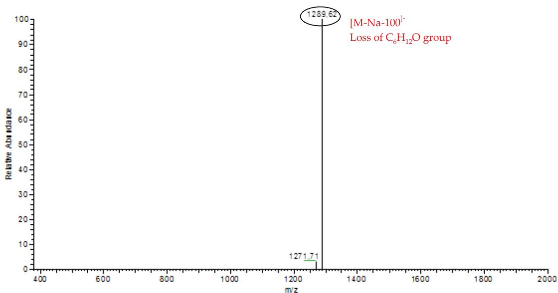
**Figure 8.** Example of a ESI-MS<sup>2</sup> spectrum, in negative mode, obtained for precursor ion  $m/z$  1389.6. In this figure it is possible to detect a mass difference of 100 Da between the precursor and the fragment ion  $m/z$  1289.6.
