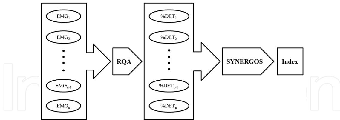
**Figure 1.** The schematic view of the SYNERGOS algorithm. EMG signals are analyzed using the RQA and the output, % DET for each muscle is imported into the SYNERGOS algorithm which eventually provides a single scalar index representing the state of MMA.
