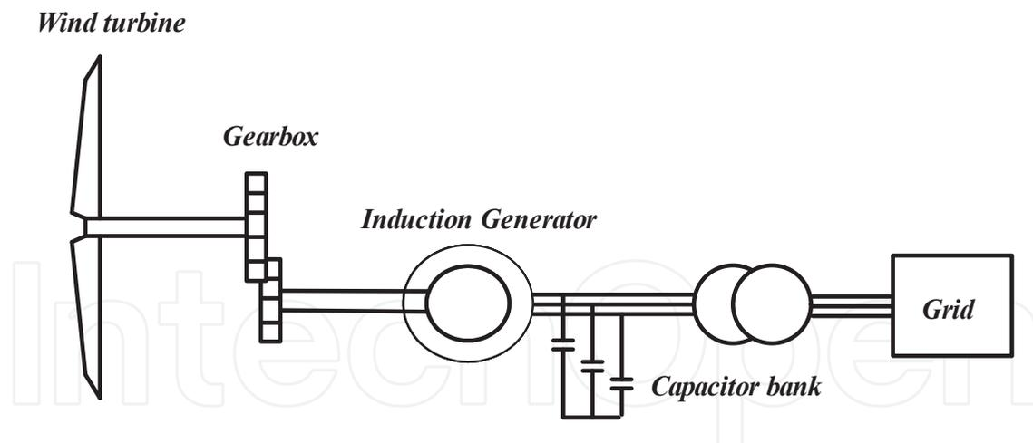
**Figure 2.** Fixed speed induction generator
