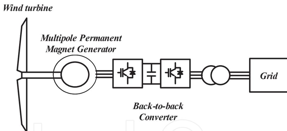
**Figure 4.** Converter-driven generator
