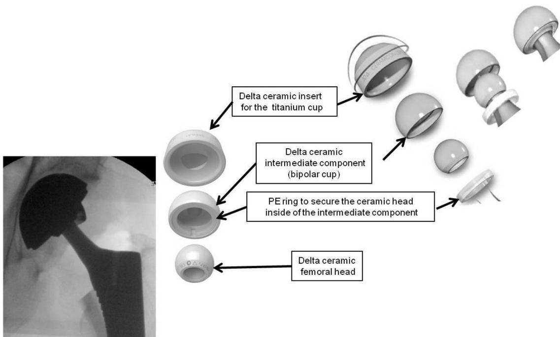
**Figure 1.** Tripolar hip prostheses have two bearing surfaces: the outer bearing surface, between the acetabular cup and the intermediate component (bipolar head), and the inner bearing surface, between the intermediate component and the femoral head component
