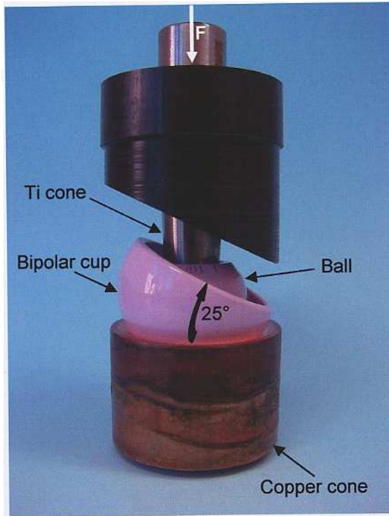
**Figure 5.** Experimental protocol for burst tests on tripolar delta ceramic (TDC) implants.
