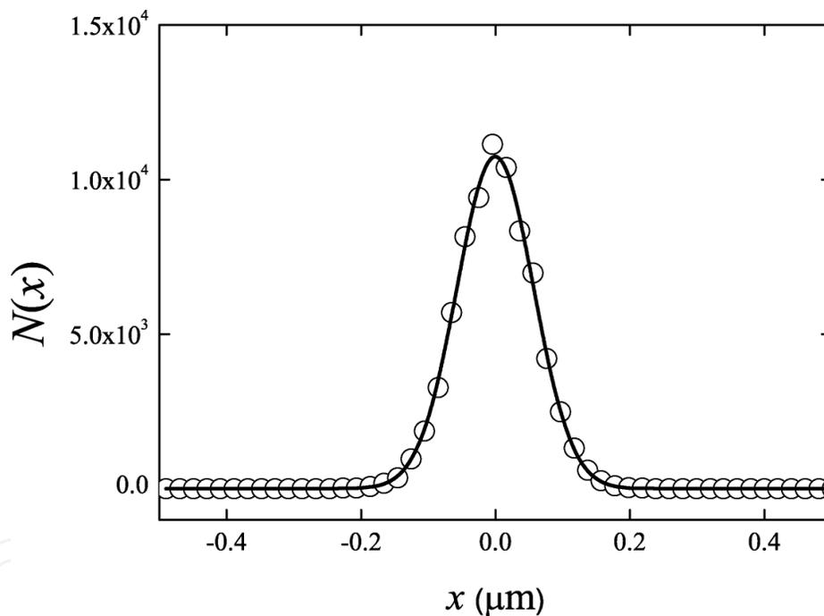
**Figure 2.** A Van Hove plot measured for 505nm polystyrene fluorescence particles diffusing in a glycerol water mixture, a homogenous medium, as can be seen by a good agreement to a Gaussian fit (solid line). Data obtained using a CMOS camera at 45Hz.
