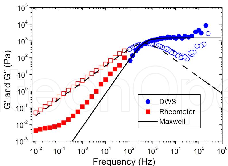
**Figure 7.** Elastic modulus  $G'$  and loss modulus  $G''$  as a function of frequency for a 30 wt% dextran (500 kDa) in water solution. Experimental data are obtained by conventional rheometry and DWS. Solid lines are a fit using a Maxwell model with one element.
