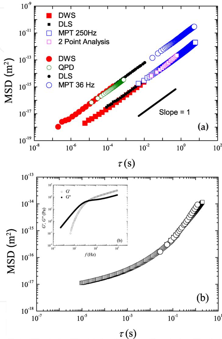
**Figure 6.** (a) Plot showing the agreement of measurements between multiple techniques in water (circles) and 62% glycerol water mixture (squares). (b) MSD plot for 4 wt% PEO showing an agreement between data obtained using DWS MPT and 2 point analysis (Inset: Extracted rheological properties).
