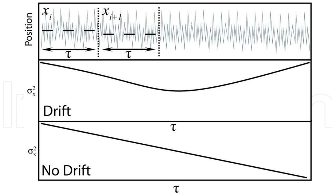
**Figure 3.** Schematic showing the relation between a particles mean position and the Allan Variance. It can be seen that in a perfect experiment, with no drift, the Allan variance decreases for the duration of the experiment, but where drift is present the Allan variance has a minimum corresponding to when the effects of sampling statistics and drift are balancing out.
