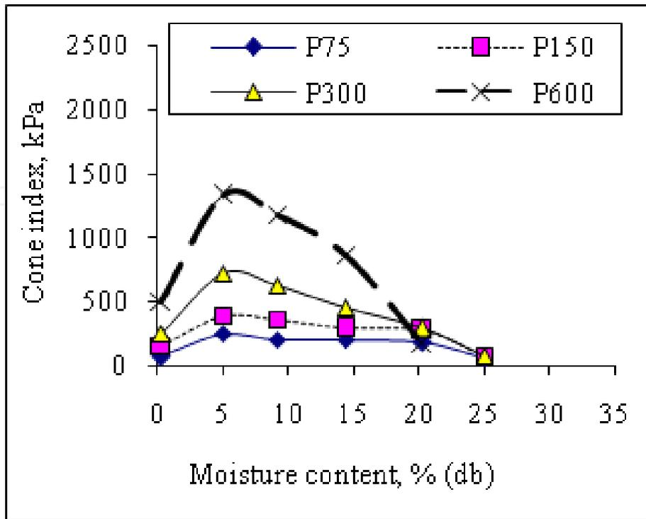
Figure 5. Effect of moisture content and applied pressure on cone index
