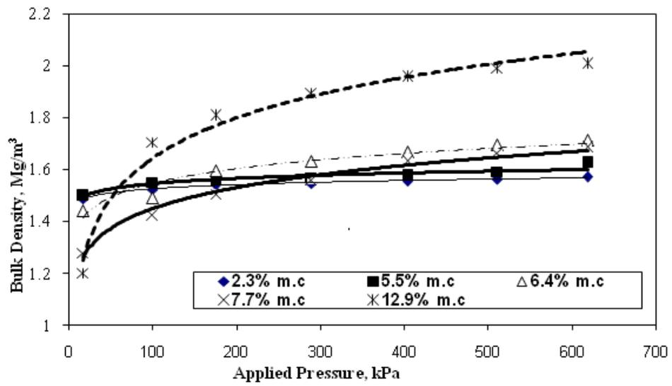
**Figure 3.** Effect of applied pressure, moisture content on bulk density of sandy clay loam soil (EBS3), Layer3 (52, 17, 31)
