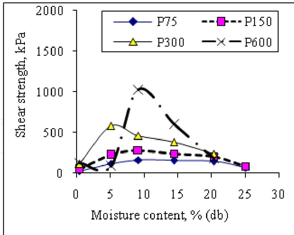
**Figure 4.** Effect of moisture content and applied pressure on shear strength
