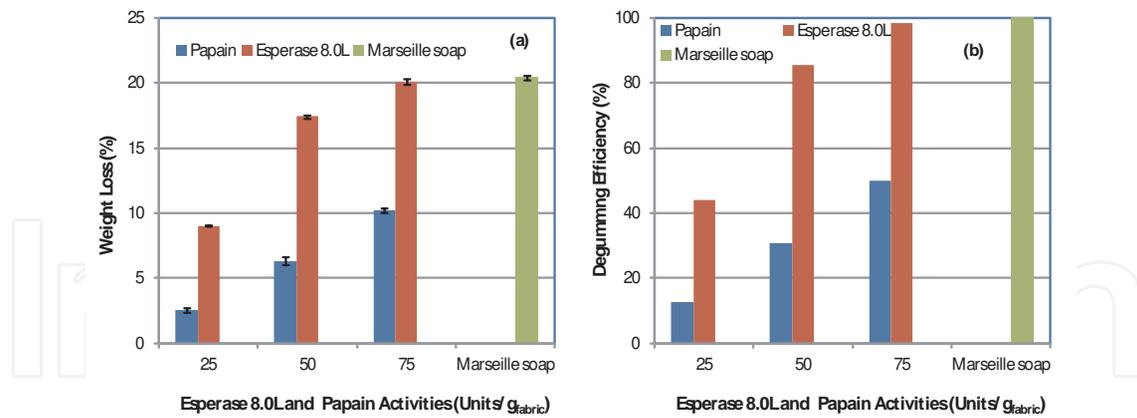
**Figure 2.** a) weight loss of silk fabrics treated with different types of proteases at enzyme dosages ranged from 25 to 74  $\text{U g}^{-1}_{\text{fabric}}$  and (b) degumming efficiency of the enzymatic process
