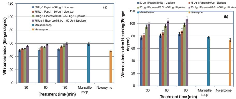
**Figure 5.** a) Whiteness Index and (b) Whiteness Index after bleaching with  $\text{H}_2\text{O}_2$  of degummed silk fabrics using Marseille soap (conventional treatment) or mixture of papain and Esperase® 8.0L with Lipolase® Ultra 50T at different loadings and treatment times.
