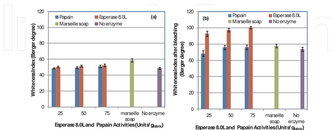
**Figure 3.** a) Whiteness Index and (b) Whiteness Index after bleaching with H<sub>2</sub>O<sub>2</sub> of degummed silk fabrics using Marseille soap (conventional treatment) or papain and Esperase® 8.0L at different loadings.
