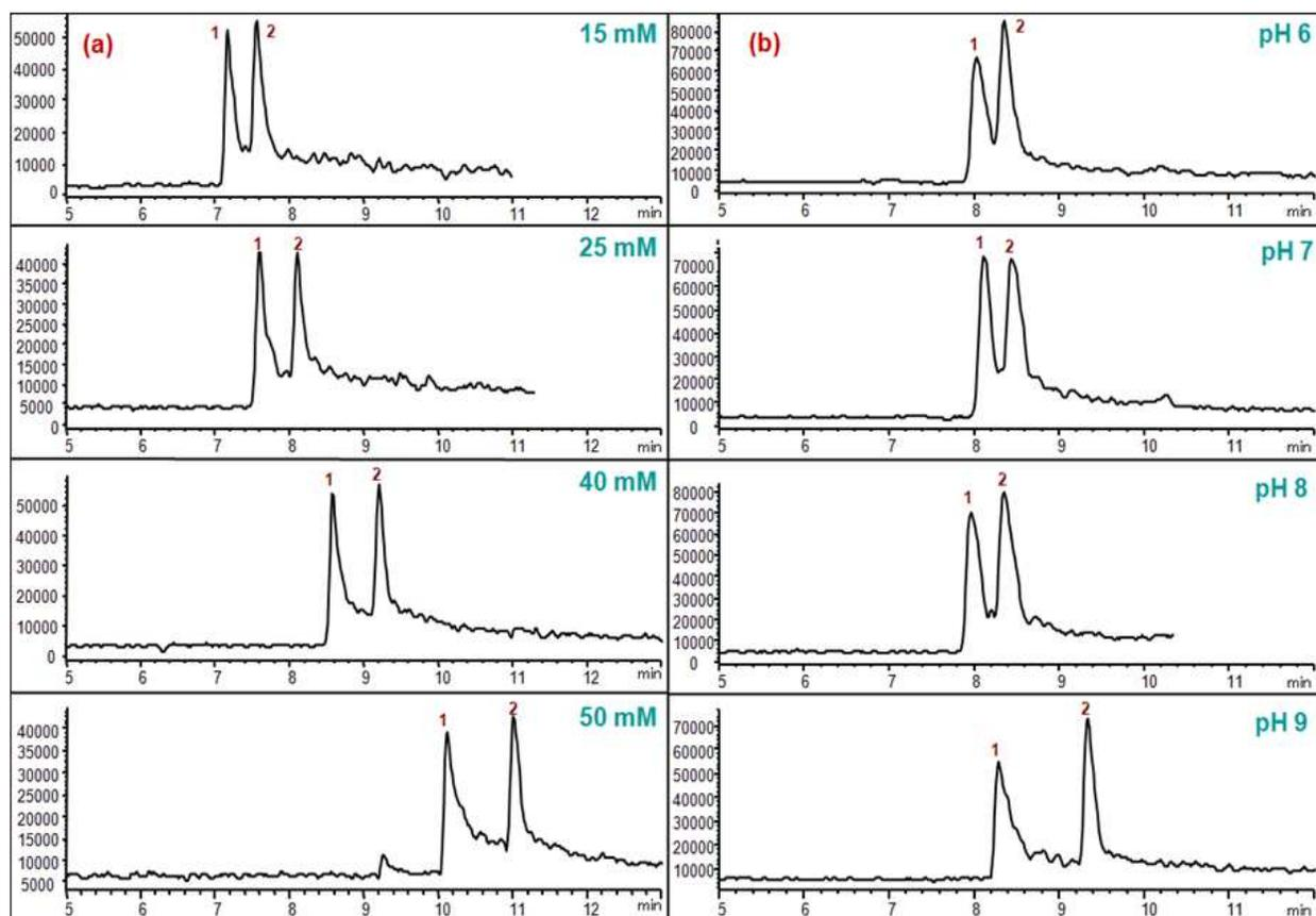
**Figure 3.** Effect of (a) ionic strength and (b) pH of the BGE on the separation of rivastigmine (2) and I.S. (1). Conditions: BGE: ammonium acetate, sheath liquid 1 % acetic acid in water:MeOH (50:50 v/v) at a flow rate of 10  $\mu$ L/min, analyte and I.S. concentrations 0.3 mg/mL. Drying gas flow rate 6 L/min and temperature 200  $^{\circ}$ C, nebulizer gas pressure 20 psi [24].
