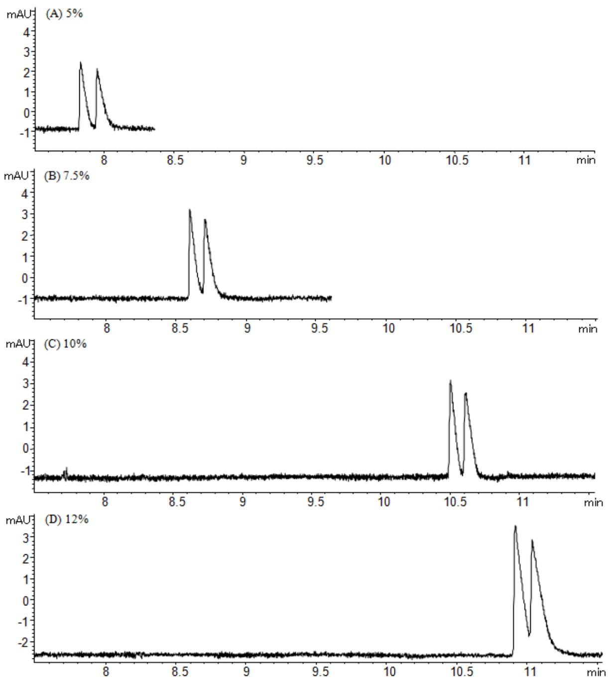
**Figure 9.** Effect of the concentration of tert-butanol on the separation of the enantiomers of Huperzine A: (A) 5%, (B) 7.5%, (C) 10% and (D) 12% (v/v). Separation conditions: BGE: 50 mM sodium acetate (pH 5.0), 0.2% (w/v) poly-LL-SUAV; pressure injection, 30 mbar for 3 s; applied voltage, 20 kV; temperature, 25 °C; fused-silica capillary, 64 cm (55.5 cm effective length) x 50  $\mu$ m i.d.; detection, 230 nm [55].
