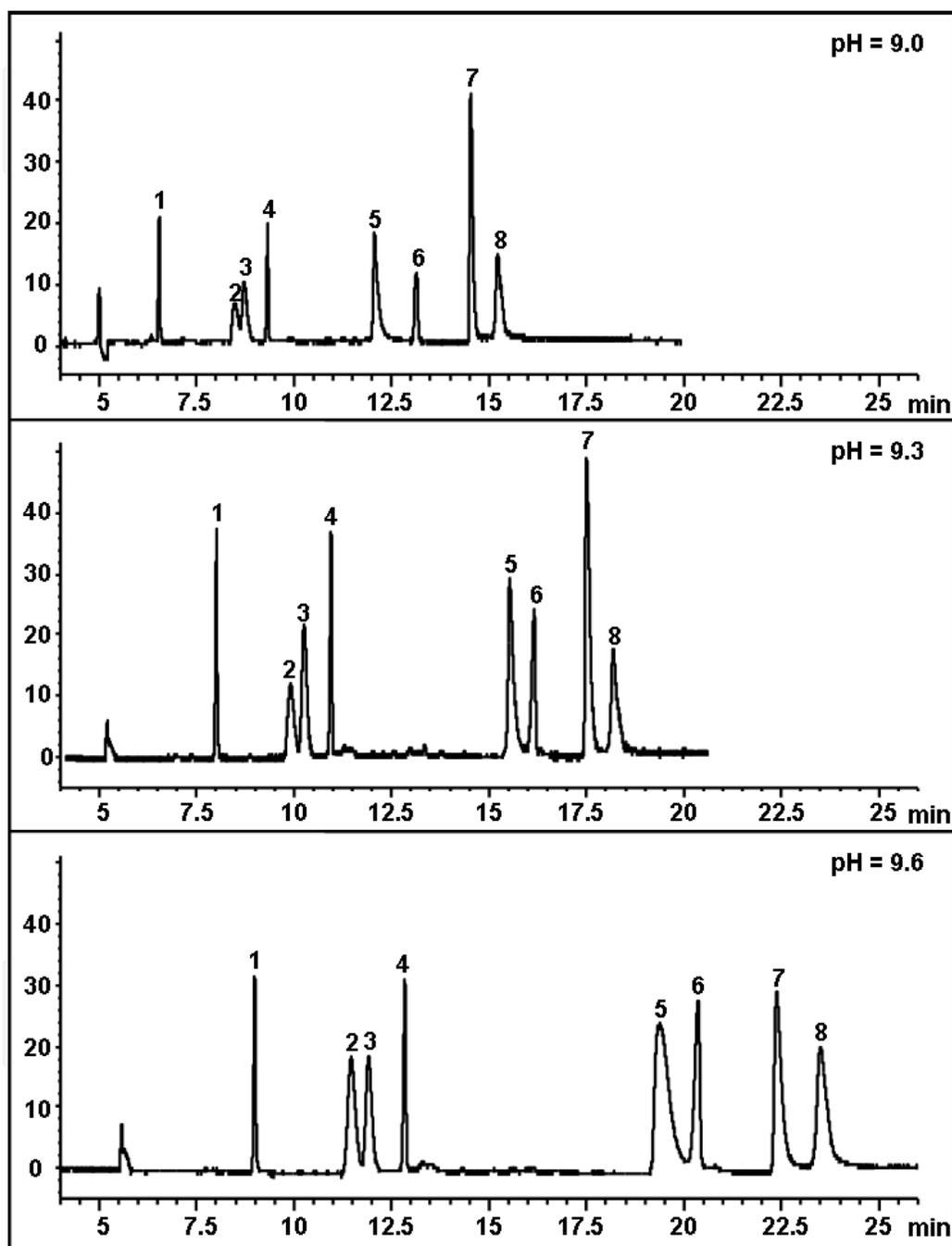
**Figure 1.** Effect of pH value on the separation of the eight polyphenols. (A) pH 9; (B) pH 9.3; (C) pH 9.6. Conditions: BGE 50 mM borate, 10 mM phosphate and 20 mM SDS; pressure injection, 30 mbar for 3 sec; applied voltage, 25 kV; temperature, 25 °C; fused-silica capillary, 64 cm (55.5 cm effective length) x 50 µm i.d.; detection, 205 nm. Peak identification: trans-resveratrol (1), epicatechin (2), catechin (3), naringenin (4), kaempferol (5), apigenin (6), myricetin (7), quercetin (8) [17].
