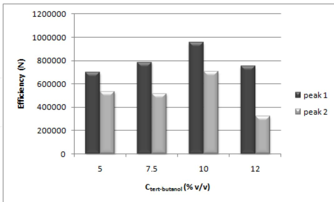
**Figure 10.** Effect of the concentration of tert-butanol on the efficiency. Separation conditions: Same as Fig. 4. BGE: 50 mM sodium acetate (pH 5.0), 0.2% (w/v) poly-LL-SUAV; pressure injection, 30 mbar for 3 s; applied voltage, 20 kV; temperature, 25 °C; fused-silica capillary, 64 cm (55.5 cm effective length) x 50  $\mu\text{m}$  i.d.; detection, 230 nm [55].
