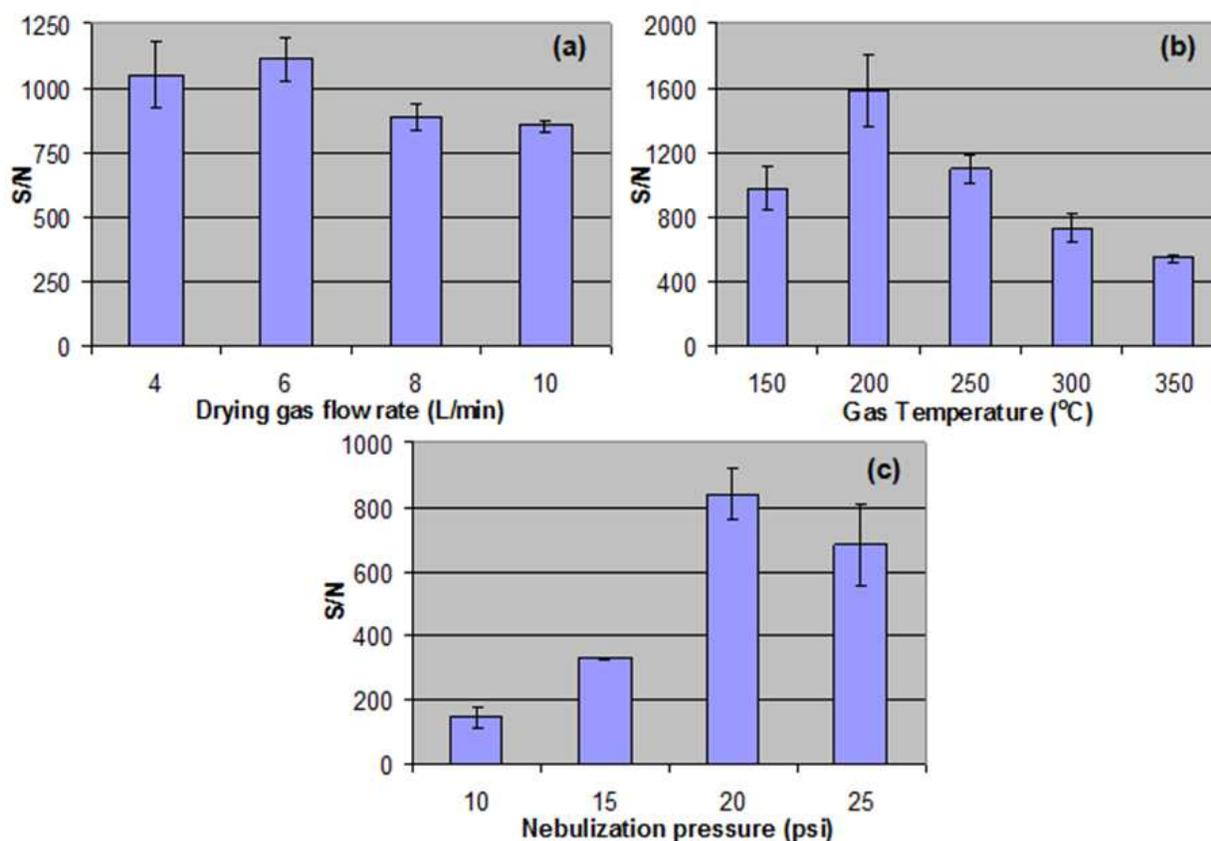
**Figure 6.** Effect of (a) drying gas flow rate, (b) drying gas temperature and (c) nebulizer gas pressure upon S/N ratio. Conditions: BGE: ammonium acetate 40 mM at pH 9.0, sheath liquid 1 % acetic acid in water:MeOH (50:50 v/v) at a flow rate of 10  $\mu$ L/min, analyte and I.S. concentrations 0.3 mg/mL [24].
