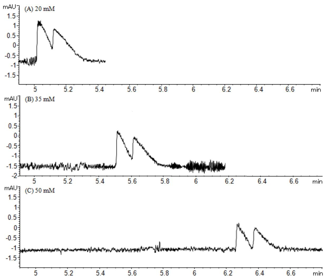
**Figure 8.** Effect of BGE concentration on the separation of the enantiomers of Huperzine A: (A) 20 mM, (B) 35 mM and (C) 50 mM. Separation conditions: BGE: sodium acetate (pH 5.0), 0.075% (w/v) poly-LL-SULV; pressure injection, 30 mbar for 3 s; applied voltage, 20 kV; temperature, 25 °C; fused-silica capillary, 64 cm (55.5 cm effective length) x 50  $\mu$ m i.d.; detection, 230 nm [55].
