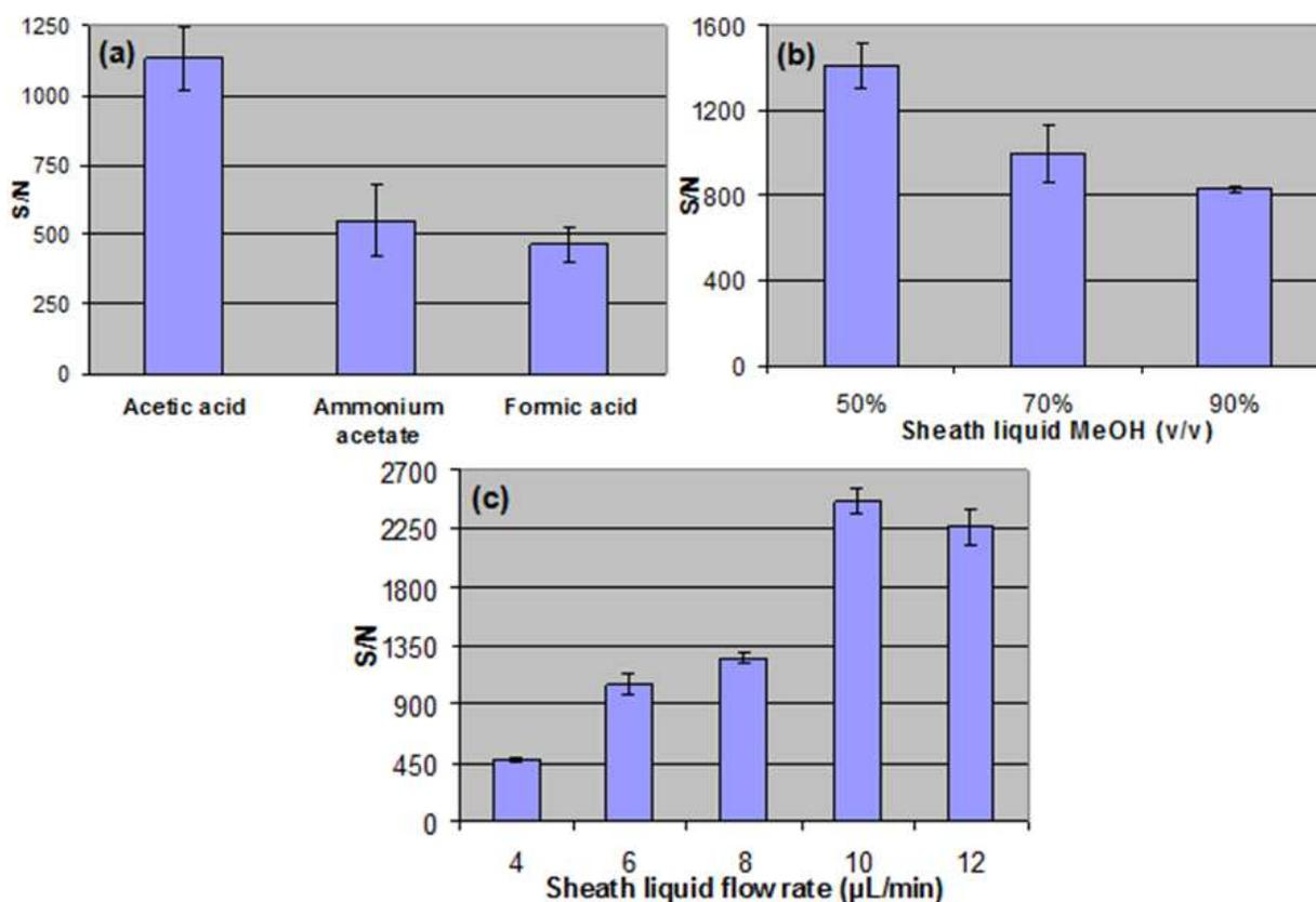
**Figure 5.** Effect of (a) sheath liquid composition, (b) sheath liquid organic modifier and (c) sheath liquid flow rate upon S/N ratio. Conditions: BGE: ammonium acetate 40 mM, at pH 9.0; analyte and I.S. concentrations 0.3 mg/mL. Drying gas flow rate 6 L/min and temperature 200 °C, nebulizer gas pressure 20 psi [24].
