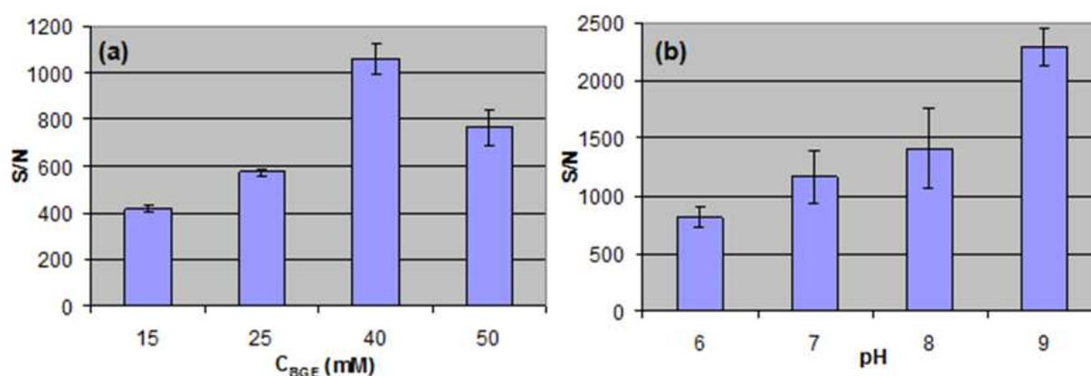
**Figure 4.** Effect of (a) ionic strength of the BGE and (b) pH of the BGE upon S/N ratio. Conditions: BGE: ammonium acetate, sheath liquid 1 % acetic acid in water:MeOH (50:50 v/v) at a flow rate of 10  $\mu$ L/min, analyte and I.S. concentrations 0.3 mg/mL. Drying gas flow rate 6 L/min and temperature 200  $^{\circ}$ C, nebulizer gas pressure 20 psi [24].
