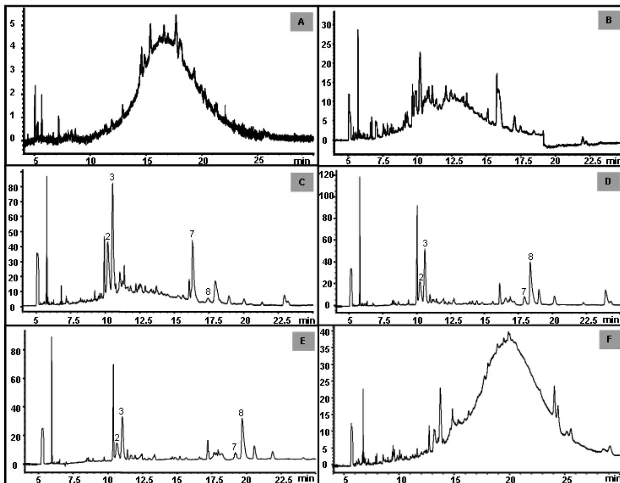
**Figure 2.** Electropherograms of the wine samples obtained using six different sample preparation procedures under optimum conditions. Conditions: BGE 50 mM borate, 10 mM phosphate and 20 mM SDS (pH 9.6); pressure injection, 30 mbar for 3 sec; applied voltage, 25 kV; temperature, 25 °C; fused-silica capillary, 64 cm (55.5 cm effective length) x 50  $\mu$ m i.d.; detection, 205 nm. Peak identification: epicatechin (2), catechin (3), myricetin (7), quercetin (8) [17].
