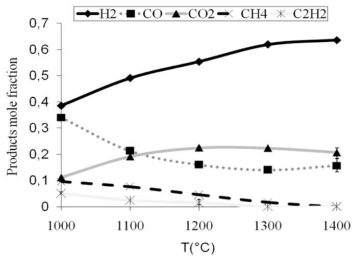
**Figure 7.** Composition of the produced syngas (dry basis and without N<sub>2</sub>) - effect of temperature, at S/F=4.5
