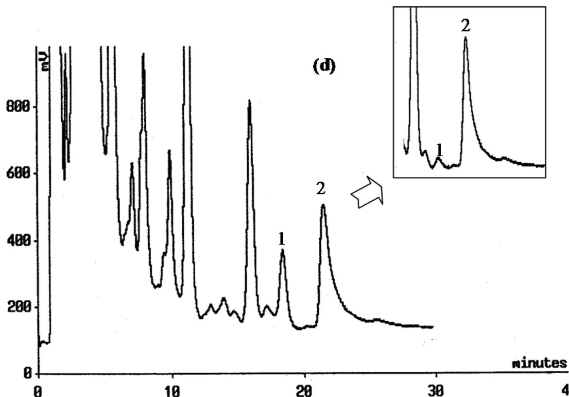
**Figure 6.** Chromatogram obtained from (a) blank reagent. (b) standard solution of (1) MPA-DNPH (10 ng/mL) and (2) P-DNPH as I.S. (c) blank of blood plasma sample, (d) blood plasma spiked with (1) MPA-DNPH (10 ng/mL) and (2) P-DNPH as I.S. (inset, (1) MPA-DNPH, 1 ng/mL).
