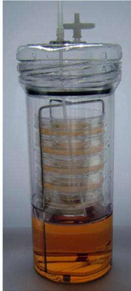
A maximum of five culture dishes (6.0 cm in diameter) can be placed on the tray of the stainless stand. The gas buffer is placed at the bottom. Two tubes protruding from the cap are inlets and outlets for gas. In-line gas filters (pore size, 0.22  $\mu\text{m}$ ) are placed at the inlets and outlets.
