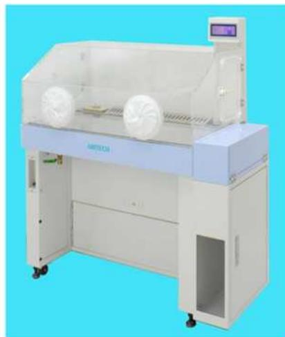
A bench top was covered with an acrylic chamber to prevent leakage of 5.0% CO<sub>2</sub>-air. Photograph A shows the system equipped with a built-in microscope, personal computer, monitor, and printer. Photograph B shows the apparatus for general handling of cultures without microscopic observation. A minimal volume of internal space is preferable for precision control of the gas phase.
