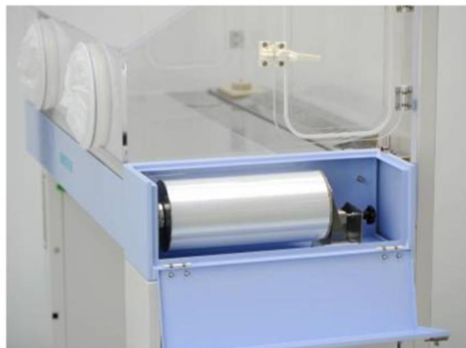
In the newly developed system, a bench top was shielded with a clear film for infection control.
