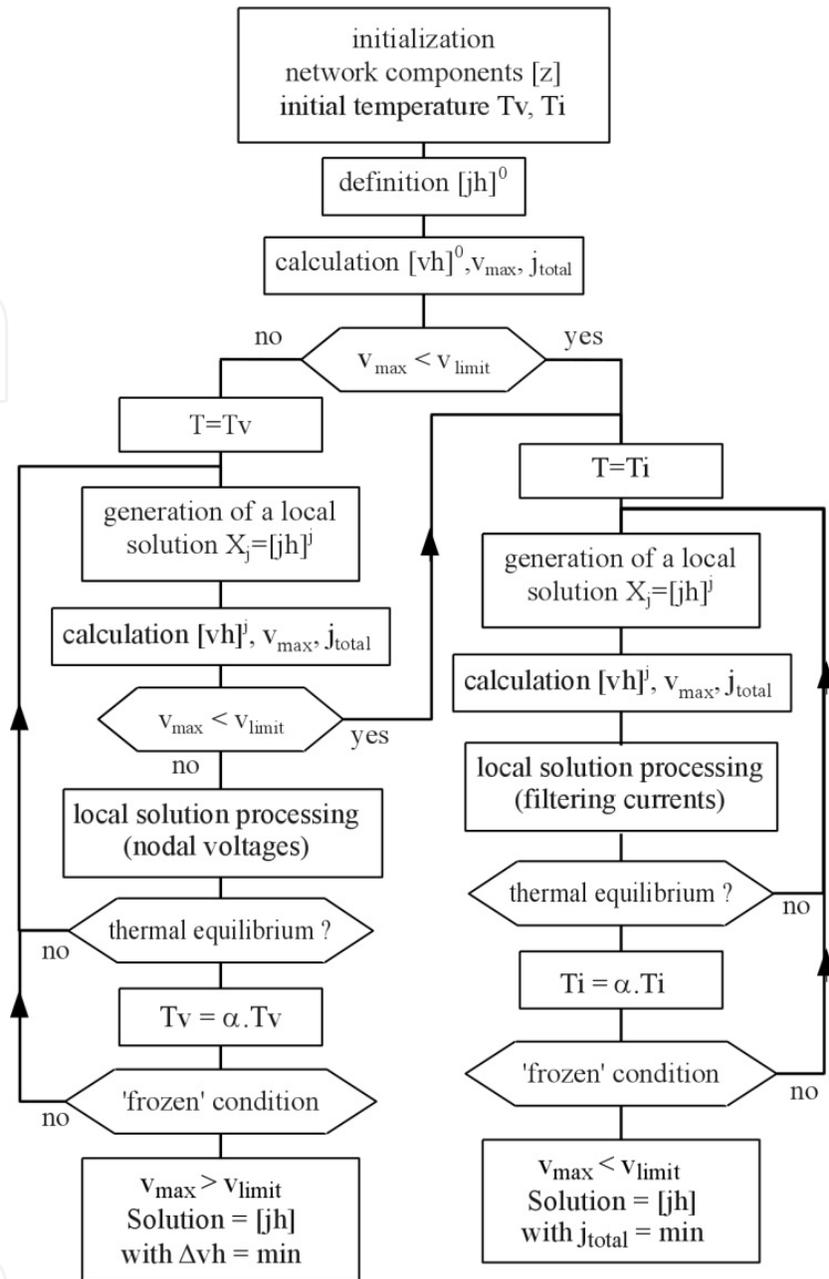
Figure 2. General flow chart of the optimisation procedure
