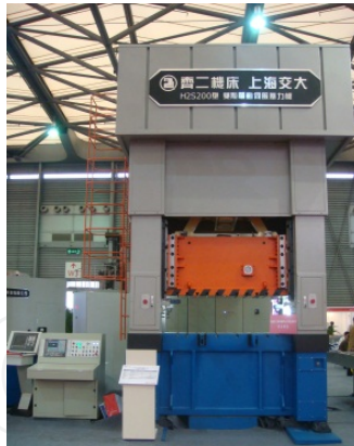
Figure 15. The servo press prototype with 2-servomotor redundant actuation of 200 tonnage (photo)
