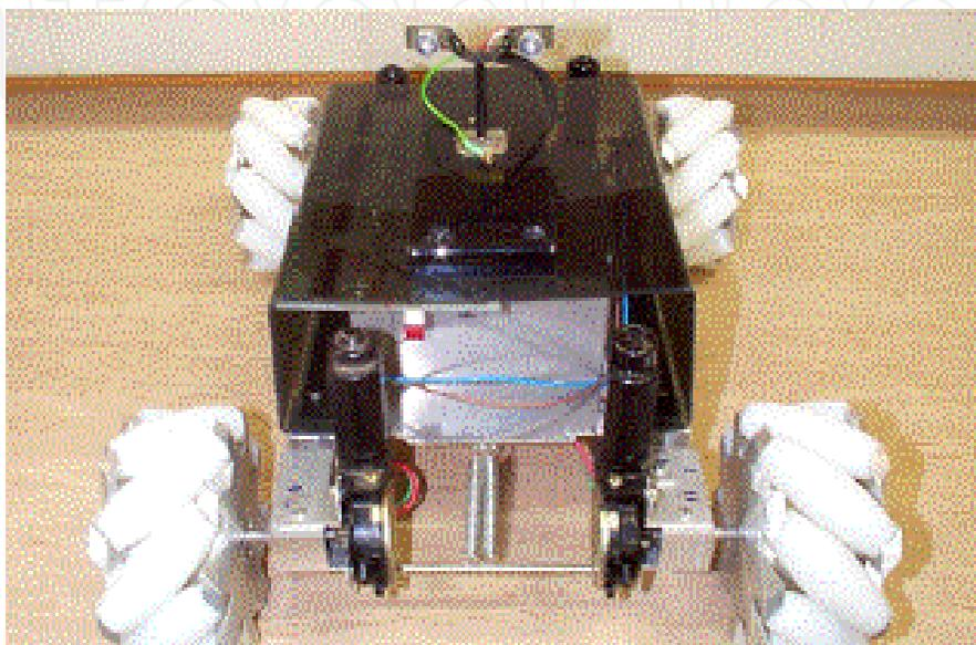
(a) Original chassis with pivot system (Phillips, 2000)
