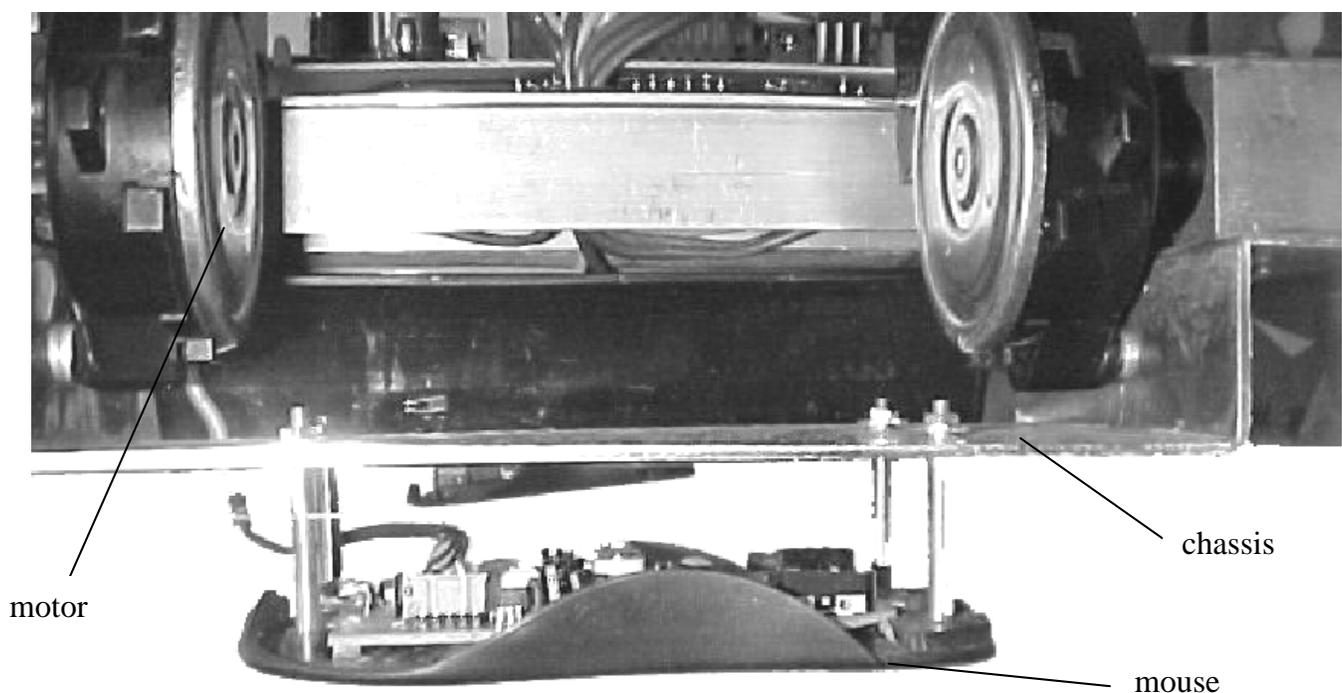
Figure 3. The Mounting of an Optical Mouse
