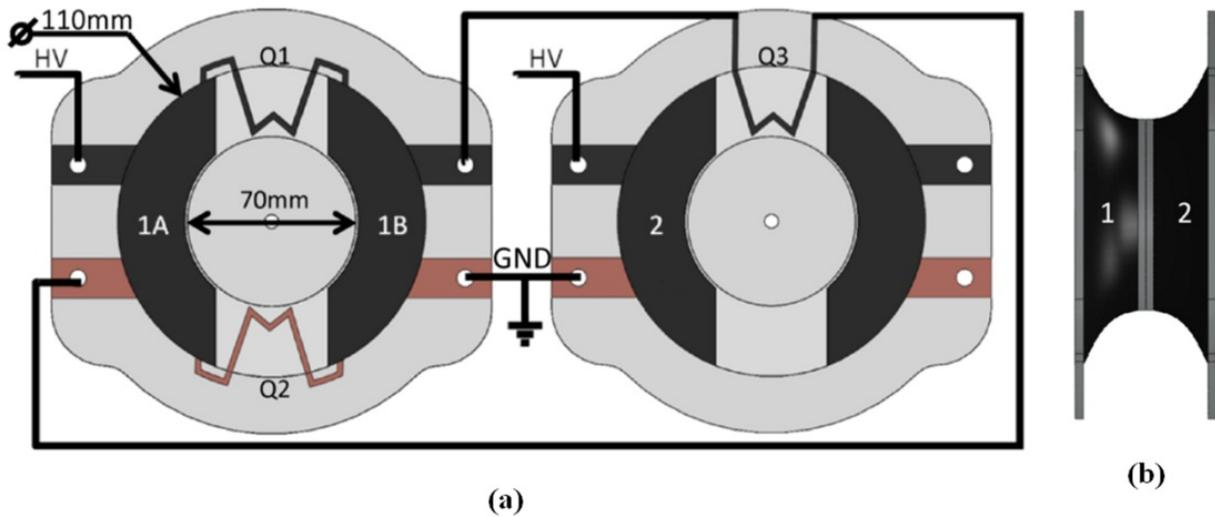
**Figure 6.** A schematic of the soft generator. The switches Q1-Q3 control the charge flow within the self-priming circuit in a similar manner to the diodes in the integrated self-priming circuit. The two diaphragms in (a) are connected together to form the antagonistic pair shown in (b). (From [24]).
