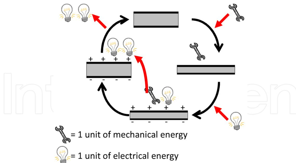
**Figure 1.** Schematic of the DEG states during a generation cycle. The grey area represents the dielectric and the black area represents the electrodes. From top moving clockwise, mechanical energy is input to the system deforming the DEG; an electrical energy input then charges the stretched DEG; the mechanical energy is then transferred to the charges by separating opposite and compressing like charges together. The electrical energy is then extracted and the cycle repeats (From [16]).
