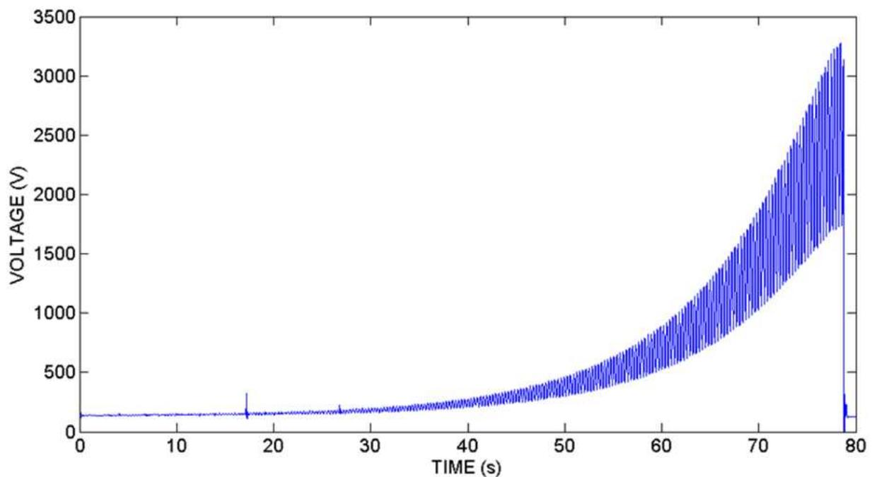
**Figure 3.** The output voltage waveform of a self-priming generator mechanically deformed at 3 Hz. The voltage climbs from cycle to cycle because the generated energy accumulates in the form of extra charge stored on the generator and priming circuit (From [19]).
