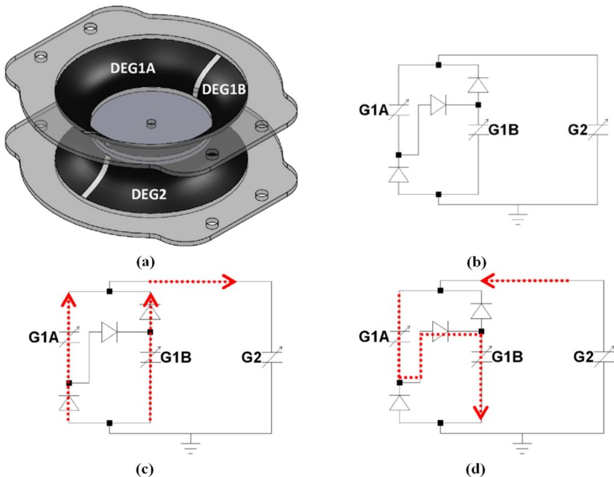
**Figure 4.** A segmented generator which consists of two membranes that are antagonistically deformed when the inner hub displaces up and down (a). The top membrane DEG1 can be electrically interconnected with diodes to form a self-priming circuit (b). The paths along which current flows off (c) and onto (d) the SPC are also illustrated.
