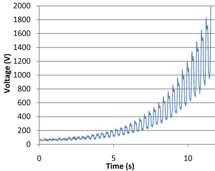
**Figure 8.** The output voltage waveform of a soft generator initially primed to 10 Volts then mechanically deformed at 3 Hz showing that the generator rapidly boosts its operating voltage through accumulation of generated energy (From [24]).
