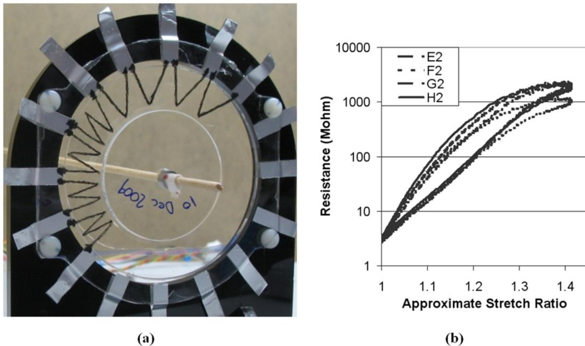
**Figure 5.** Carbon powder-based DES applied to a dielectric elastomer diaphragm (black “M” and “V” shaped tracks) for characterisation by O'Brien et al. (a), and a plot of measured DES resistance versus approximate radial stretch ratio showing that the resistance climbed several orders of magnitude when the DES were stretched (b). Images taken from O'Brien [23].
