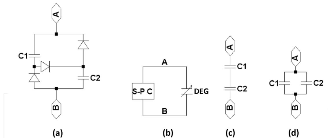
**Figure 2.** Schematic of a self priming circuit (a) which connects to a DEG in parallel (b), the diodes control current flow so that the SPC capacitor bank takes on the form given in (c) when energy is transferred to it from the DEG, when energy is transferred off the SPC the diodes configure it to take on the higher charge form given in (d).
