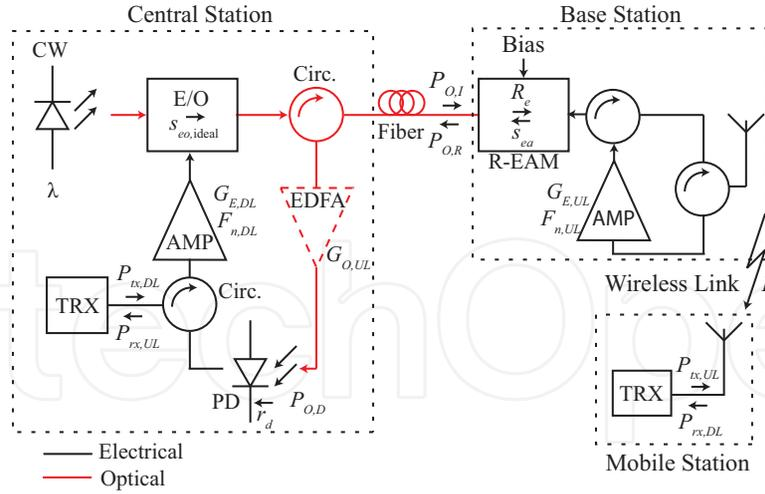
**Figure 17.** Considered setup for performance assessment. CW represents a continuous wave light source. Both TRX shown, represent the transceivers at the Control Station and Mobile Station. PD represents the Control Station photodiode. The EDFA depicted, represents an optional Erbium Doped Fiber Amplifier.
