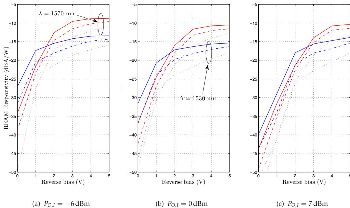
**Figure 13.** O/E response vs. reverse bias voltage for different wavelengths and frequencies and optical input powers. Solid, dashed and dotted lines correspond to frequencies of 2.4, 5, 15 GHz, respectively
