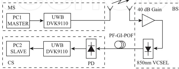
**Figure 2.** Schematic illustrating the RoF setup used.
