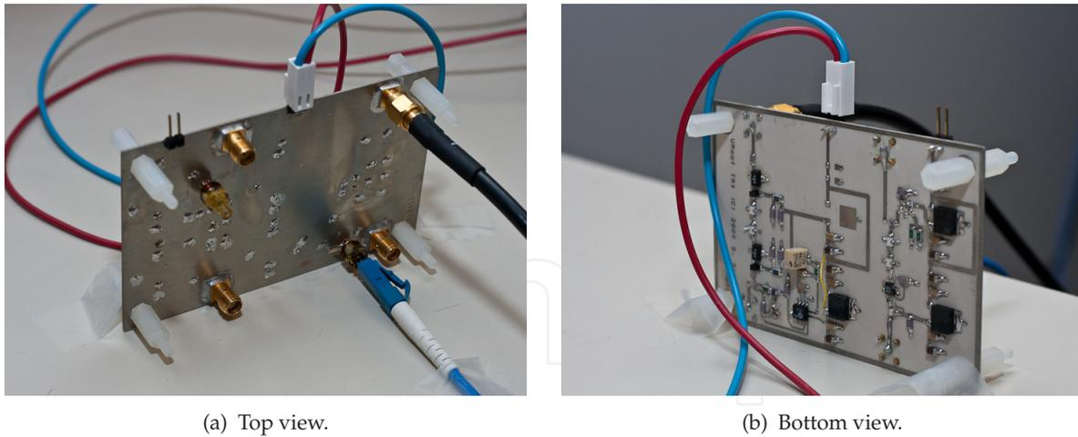
**Figure 4.** RoF conversion board used as E/O/E transceiver.
