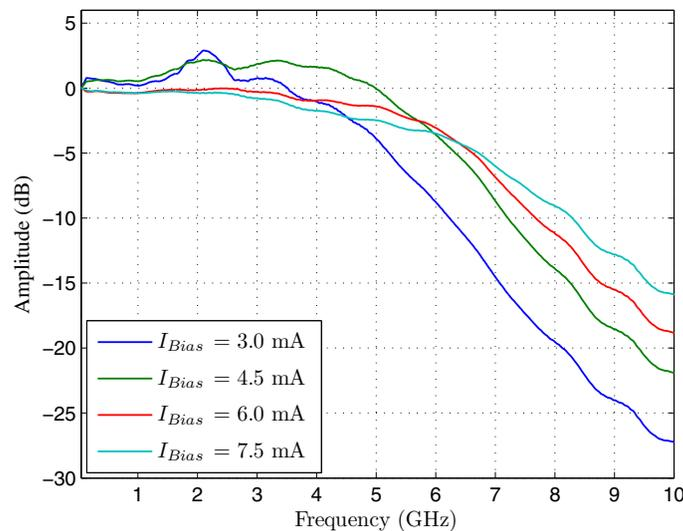
**Figure 5.** VCSEL transfer function vs. DC bias current.
