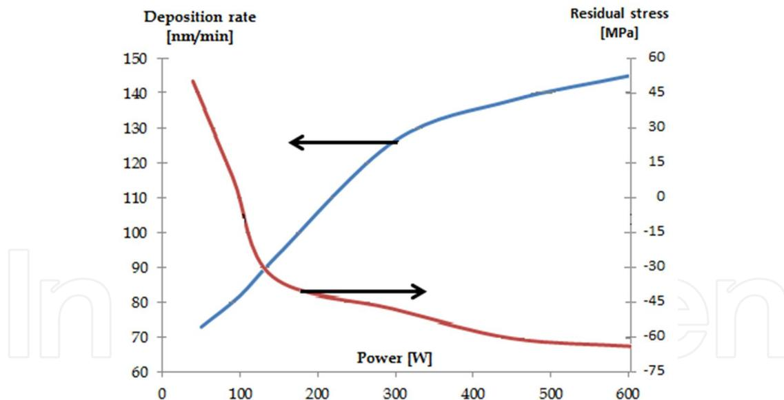
**Figure 2.** Variation of the deposition rate and residual stress with the HF power in the STS Multiplex Pro-CVD PECVD reactor. The deposition temperature was 300°C, the pressure 1100mTorr, and the gas flow rates of SiH<sub>4</sub>, CH<sub>4</sub> and Ar were 45, 300 and 700sccm, respectively.
