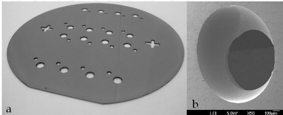
**Figure 6.** (a) Optical image of a glass wafer coated with PECVD  $\alpha$ -Si/PECVD  $\alpha$ -SiC/Photoresist after etching through in HF 49%, and (b) a SEM picture of one of the resulted etch-through holes in the glass wafer.
