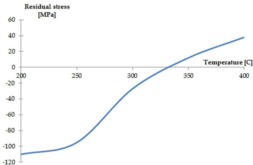
**Figure 4.** Variation of the average residual stress of PECVD  $\alpha$ -SiC films with the deposition temperature. The films were deposited in the HF mode at a power of  $150\text{W}$ , at a pressure of  $1100\text{mTorr}$ , and with gas flow rates of  $\text{SiH}_4$ ,  $\text{CH}_4$  and Ar of  $45$ ,  $300$  and  $700\text{sccm}$ , respectively.
