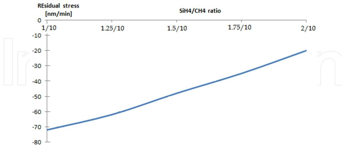
**Figure 5.** Variation of the average residual stress with the  $\text{SiH}_4/\text{CH}_4$  ratio for PECVD  $\alpha\text{-SiC}$  films deposited at  $300^\circ\text{C}$ . The  $\text{SiH}_4$  flow rate was kept constant at  $45\text{sccm}$ , while all the other deposition conditions were the same as those indicated in Fig. 4.
