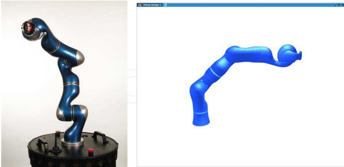
Figure 1. DLR-Lightweight-Robot-III. The picture on the right hand side shows the initial configuration of the robot in the simulation study
