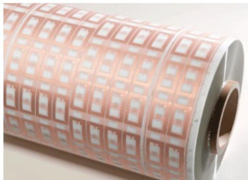
**Figure 4.** Thin foil antenna structures on a roll
