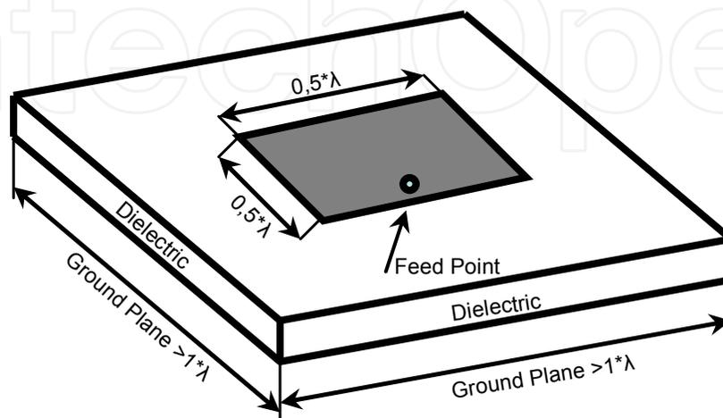
**Figure 2.** Principal structure of a squared patch antenna
