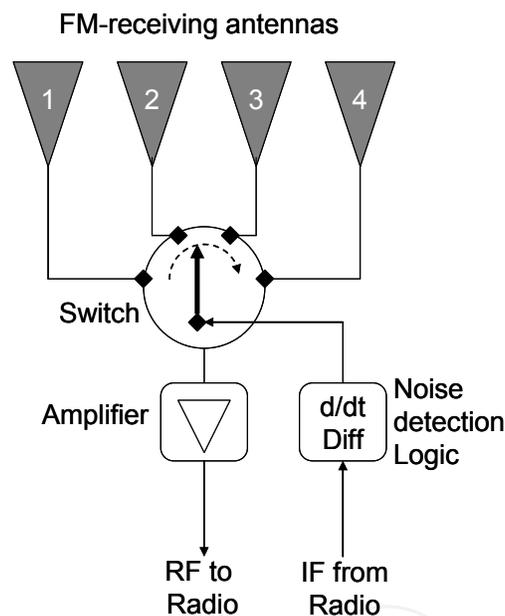
**Figure 8.** Principle of switched diversity in modern tuners [1]
