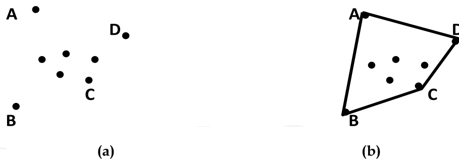
Fig. 1. (a) Input cities and (b) boundary tour formed by four extreme cities
