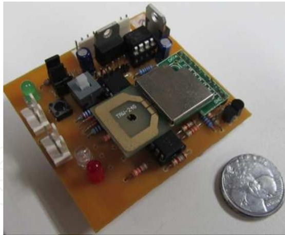
**Figure 4.** Intelligent Sensor Module - SSM.
