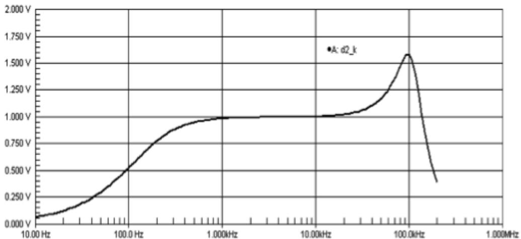
Figure 10. Frequency response of the TX amplifier.
