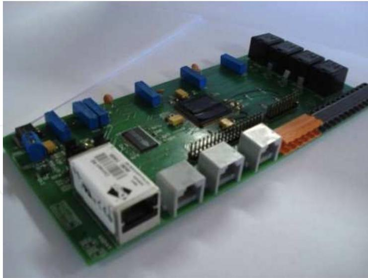
**Figure 6.** Remote Data Acquisition Unit - RDAU.
