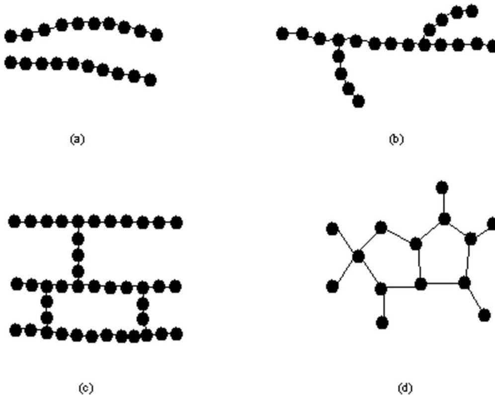
**Figure 3.** Schematic representation of: (a) linear, (b) ramified, (c) with crossed bonds and (d) network [21].
