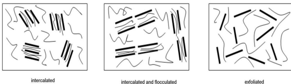
**Figure 4.** Polymer/ clay nanocomposites morphologies.
