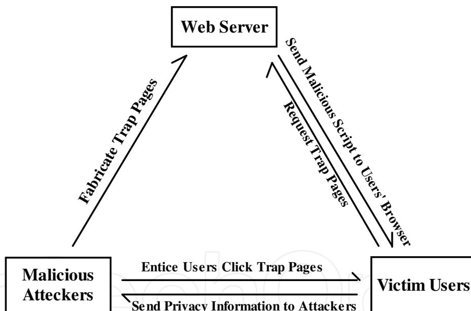
Fig. 1. The Process of Cross Site Scripting Attack
