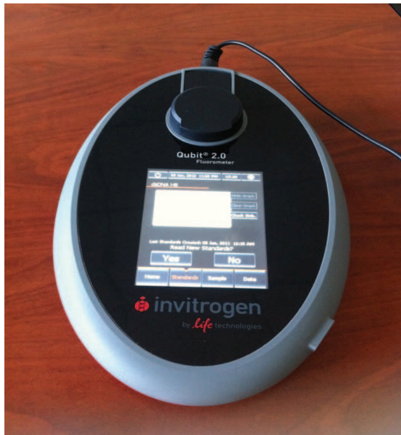
Fig. 4. QUBIT 2.0 fluorometer were used for both template DNA quantitation and the analysis of PCR products as fluorometrically
