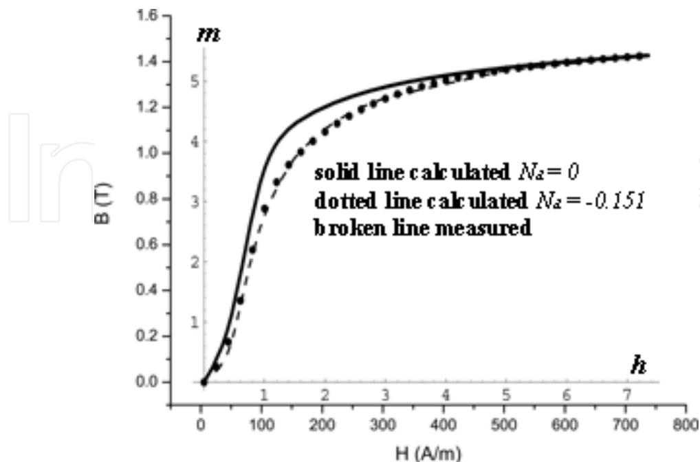
Fig. 7. Measured (broken line), modelled (dotted line) and intrinsic (solid line) loci for NO Fe-Si
