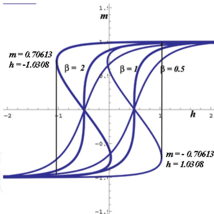
Fig. 11. Schematic hysteresis loops calculated from (42) and (43) showing the Barkhausen jump on macroscopic scales,  $\beta$  as parameter. Curves are for  $\beta = 0.5, 1$  and  $2$  in arbitrary units.
