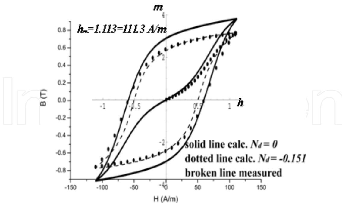
Fig. 8. Calculated NO Fe-Si minor hysteresis loop for  $N_d = 0$  (solid line) and  $N_d = -0.151$  (dotted line), fitted to the measured loop (broken line) with internal demagnetization.
