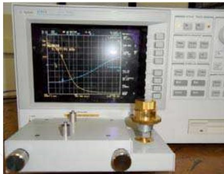
Fig. 9. Impedance meter Agilent 4294A and magnetic module
