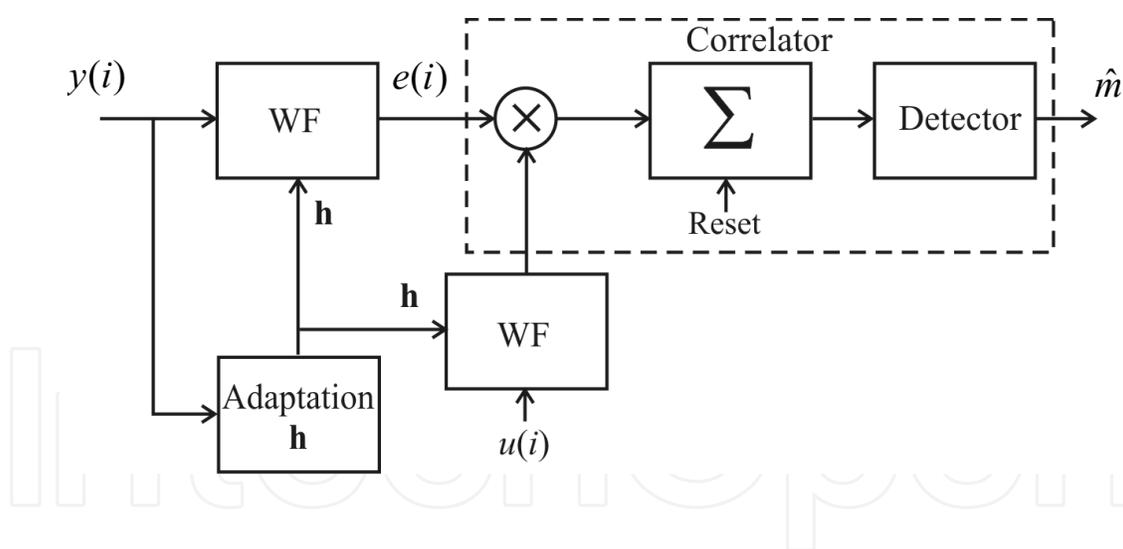
Fig. 9. Optimal receiver for watermark on the background of correlated noise
