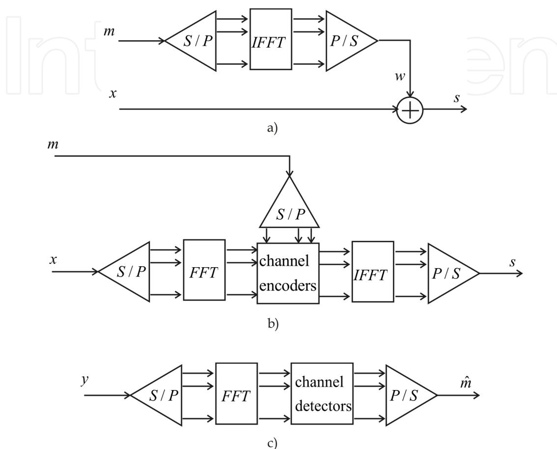
Fig. 4. OFDM application for watermarking: a) noninformed encoding; b) informed encoding; c) decoding
