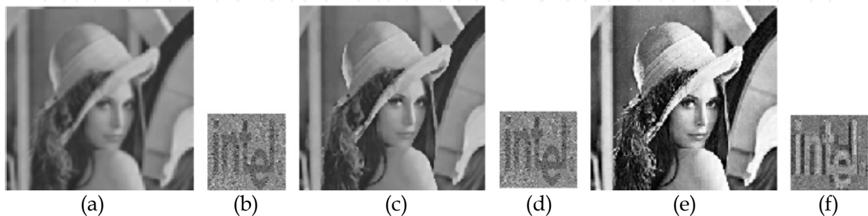
Fig. 17. (a), (c): Watermarked images after mean and median filtering, respectively, (b) and (d): Extracted watermarks from (a), and (c), respectively, (e) watermarked image after histogram equalization, (f) extracted watermark from Fig. (e).
