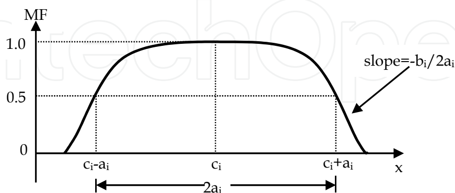
Fig. 1. Gbell shape for MF curve in input side
