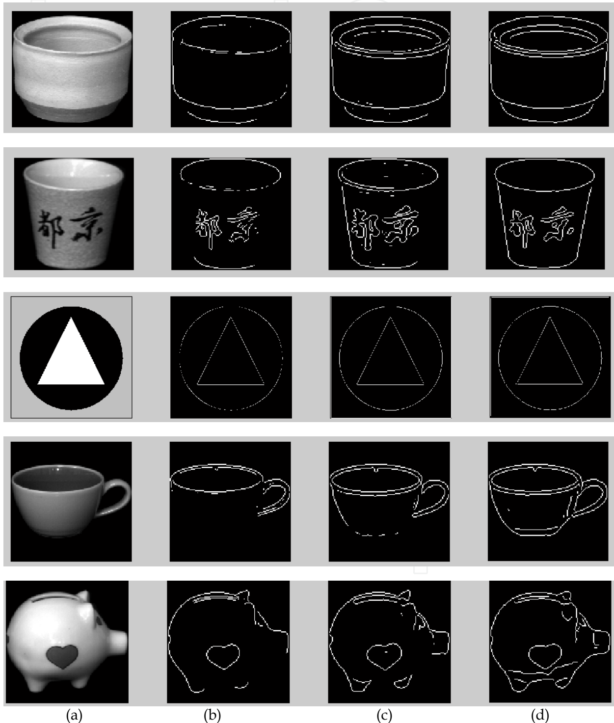
Fig. 6. Using different methods to detect the image with gradation of gray levels
