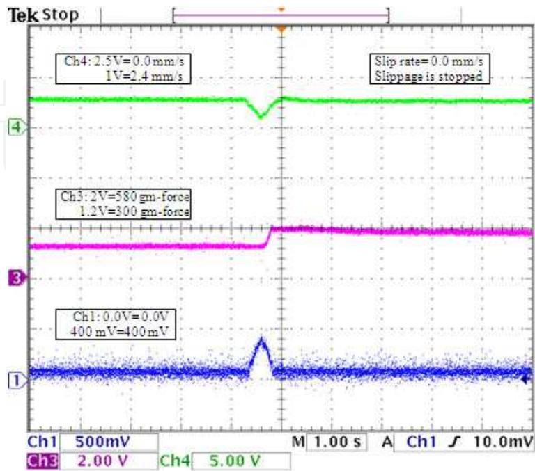
Ch4: Slip-rate (mm/s) - Ch3: Fapp (gm-force) - Ch1: Vref (V)
