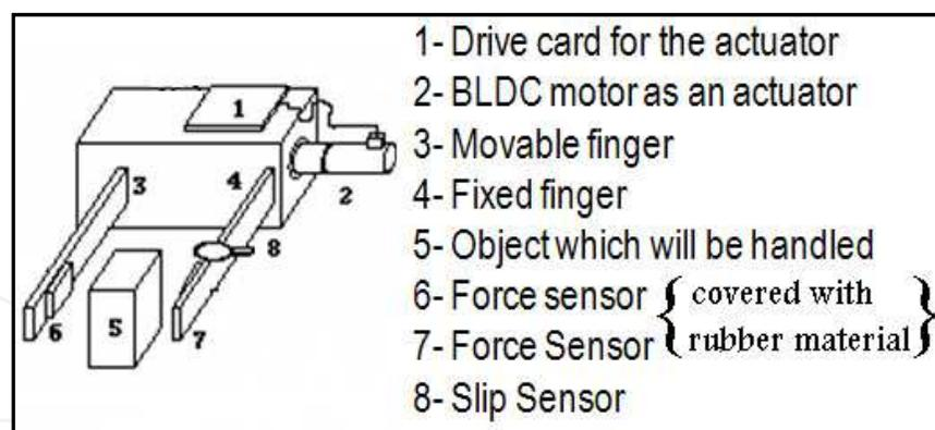
Fig. 4. Gripper configuration.
