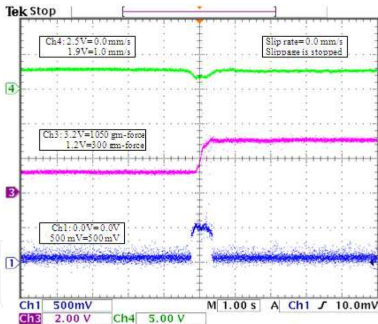
Ch4: Slip-rate (m/s) - Ch3: Fapp (gm-force) - Ch1: Vref (V)
