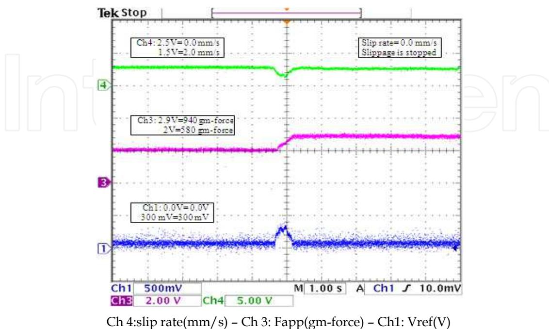
Fig. 29. System response when mass is suddenly increased from 550 to 900gm
