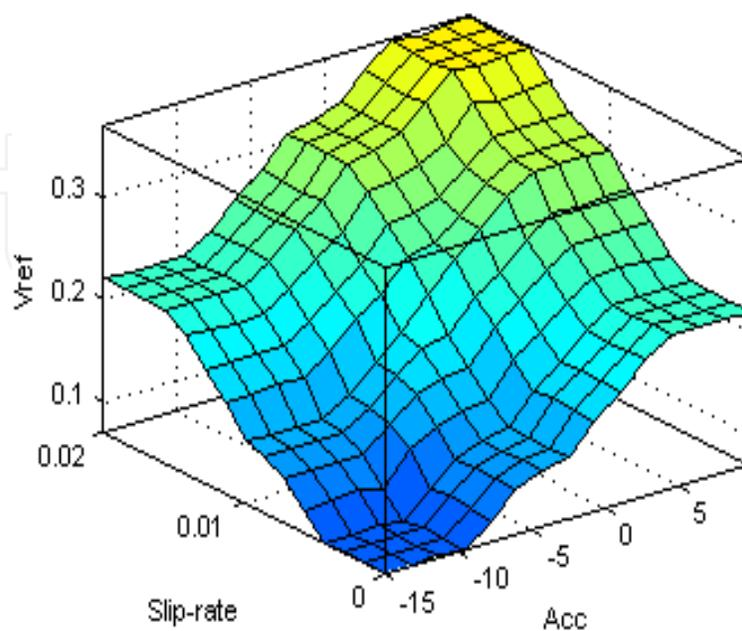
Fig. 20. Surface viewer of the reference voltage controller.
