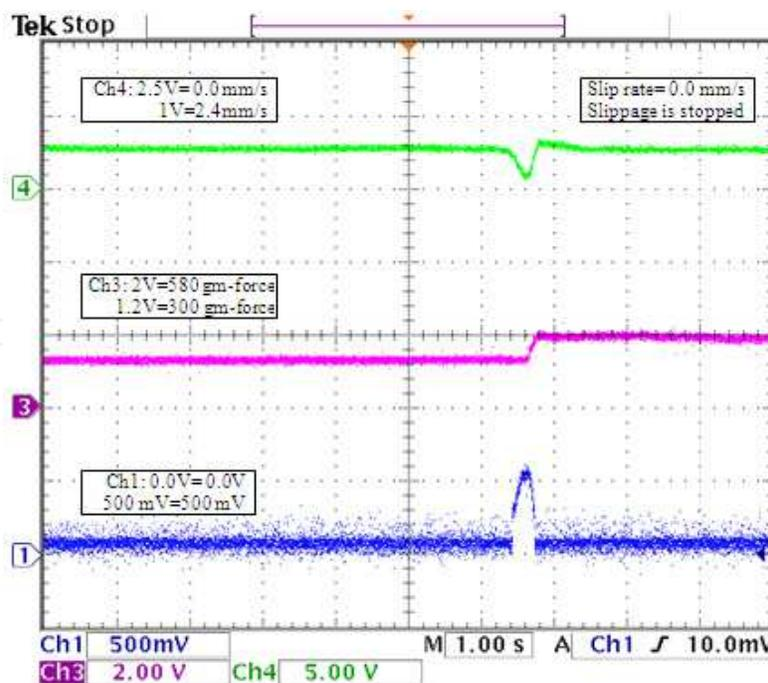
Ch4: Slip-rate (mm/s) - Ch3: Fapp (gm-force) - Ch1: Vref (V)
