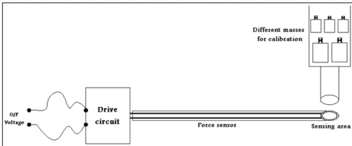
Fig. 8. Experimental test for force sensor calibration
