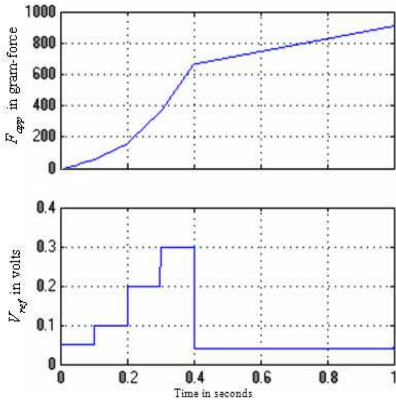
Fig. 14. Gripper simulation results using ANFIS modeling.
