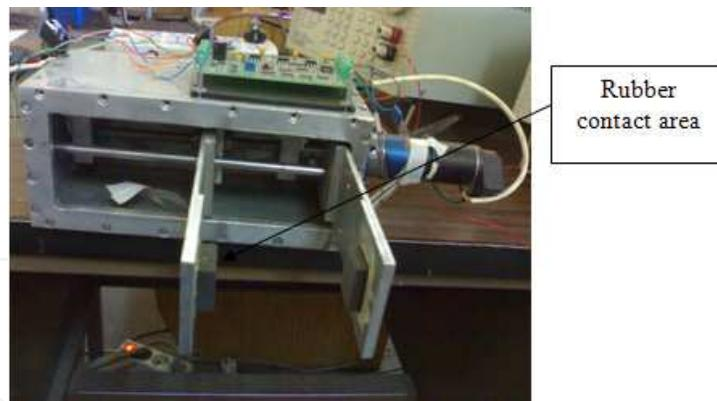
Fig. 5. Gripper prototype.
