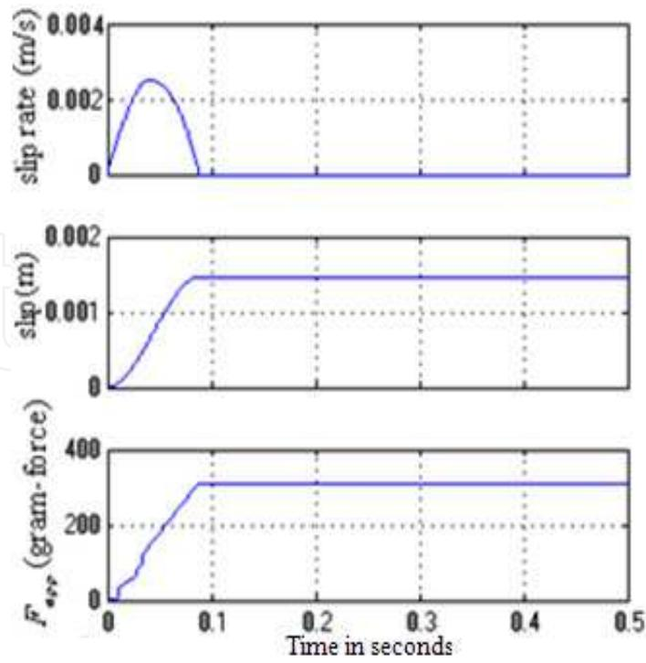
Fig. 24. System response for the second scheme controller Mass = 300 gm and  $F_{push}$  =150 g
