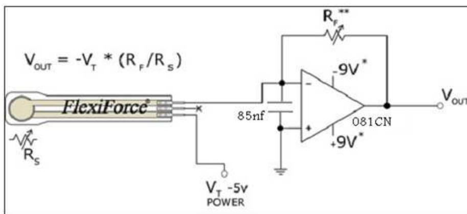
Fig. 10. Proposed drive circuit.
