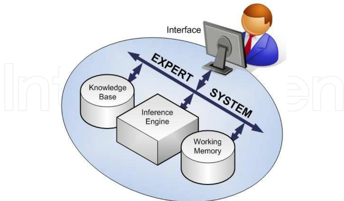
Fig. 2. Basic architecture of an Expert System
