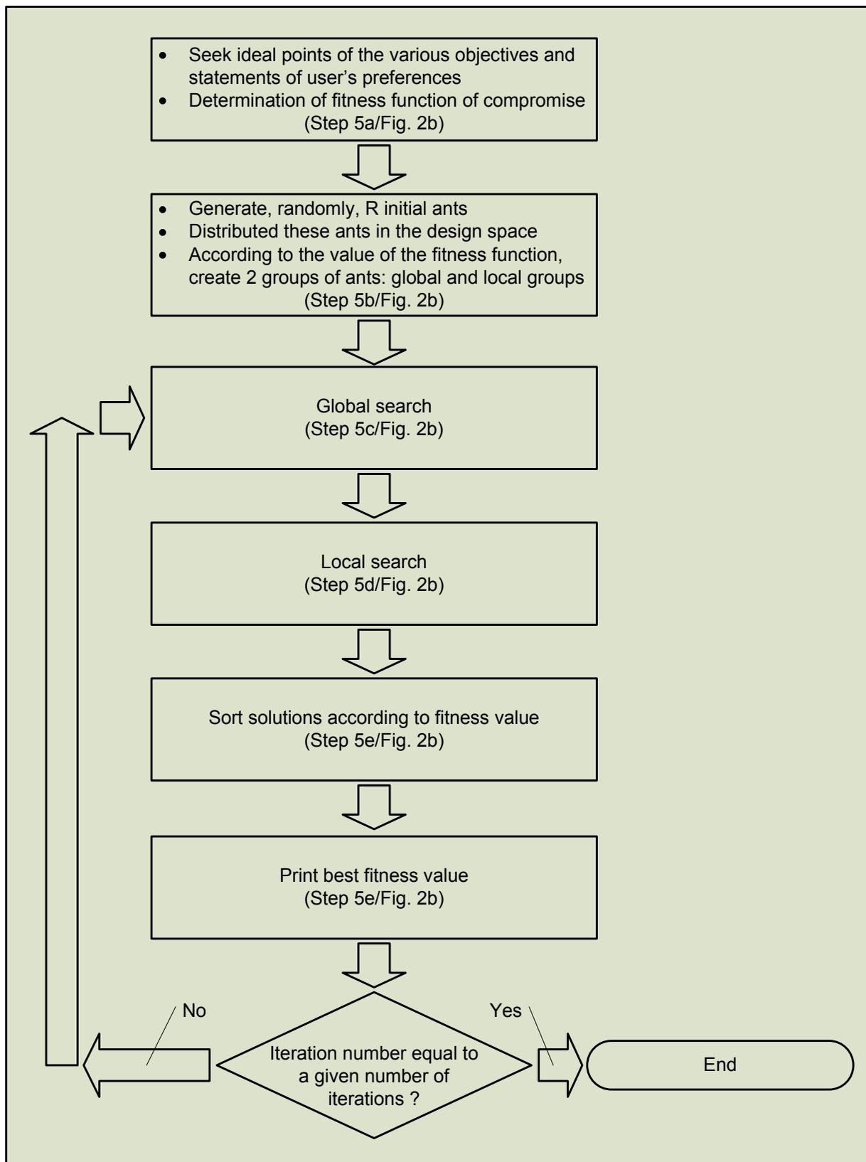
Figure 2b. Flow chart of the ACO process
