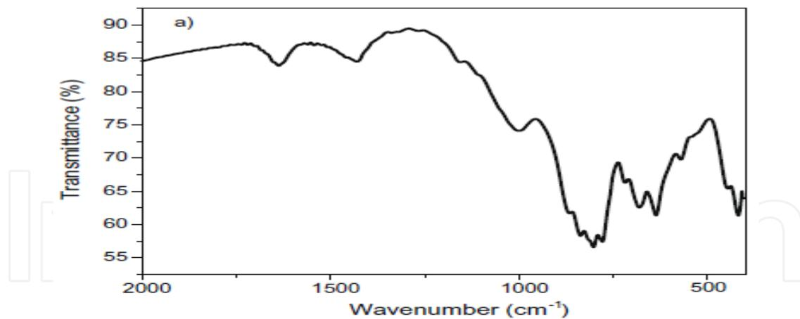
Fig. 7. IR spectra of commercial calcium aluminate cement.
