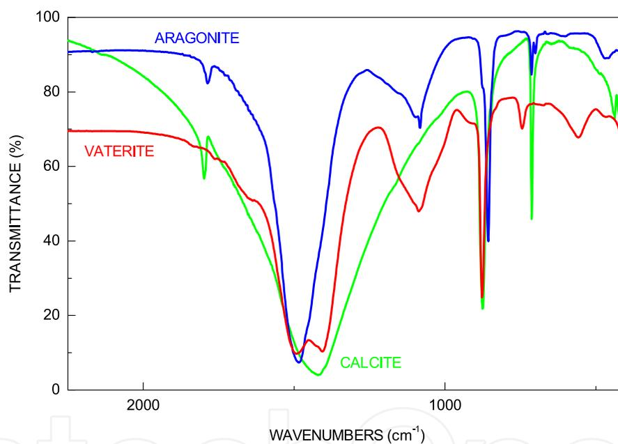
Fig. 14. Infrared spectra of calcite, vaterite and aragonite.
