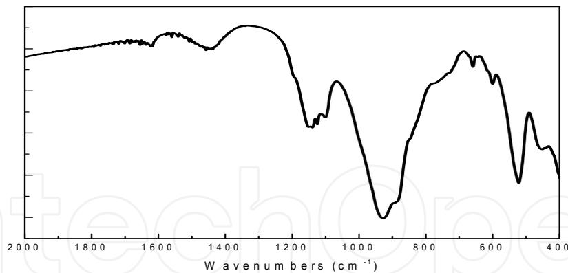
Fig. 4. IR Spectrum of ordinary Portland cement.
