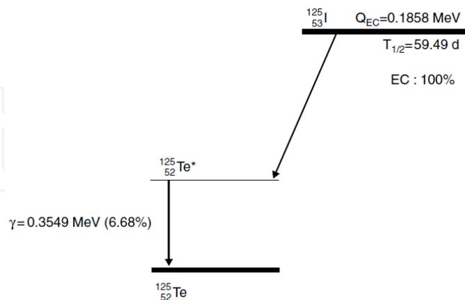
Fig. 2. Iodine-125 decay scheme [Baltas et. Al., 2006]
