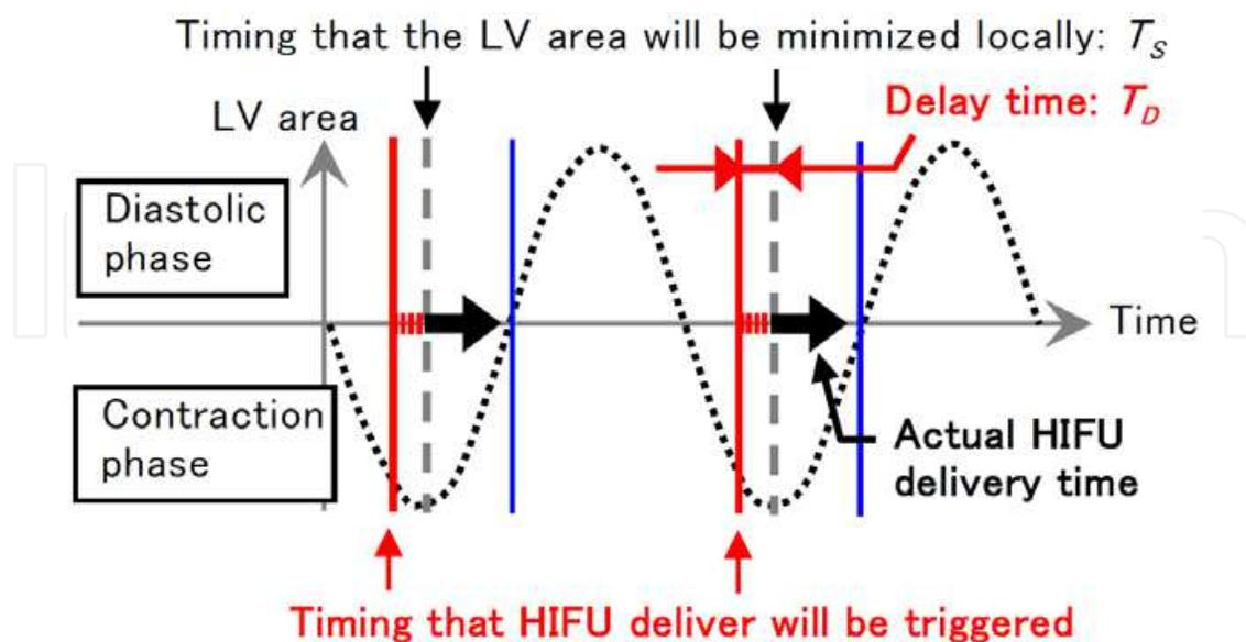
Fig. 7. Definition of HIFU delivery starting trigger timing with total delay time in the system. The timing is the delay time TD before the timing TS that the left ventricle area will be minimized locally.
