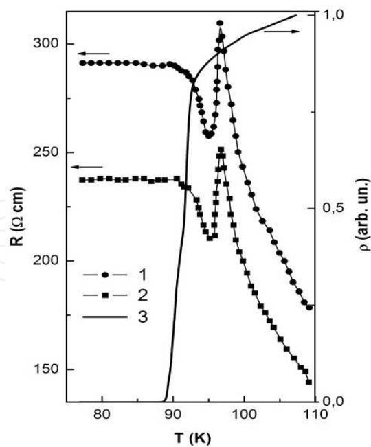
Fig. 6. Dependencies of the resistance  $R$  versus temperature for the  $\text{YBa}_2\text{Cu}_3\text{O}_{7-\delta}/\text{BiOCl:Ti}$  HCS along the semiconductor layer in (100) plane (curve 1) and trough the junction (perpendicular to (001) plane; curve 2). The curve 3 characterize the temperature dependence of  $\text{YBa}_2\text{Cu}_3\text{O}_{7-\delta}$  ceramics resistance
