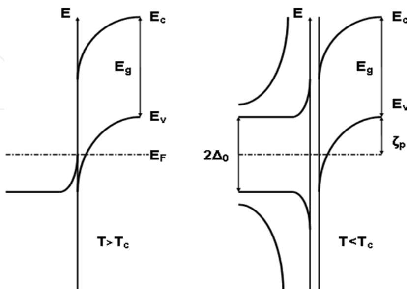
Fig. 9. The energy band diagram of “HTSC/SeC” heterojunctions
