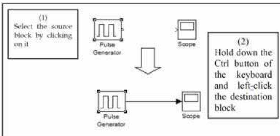
Fig. 8. Linking blocks in the model file
