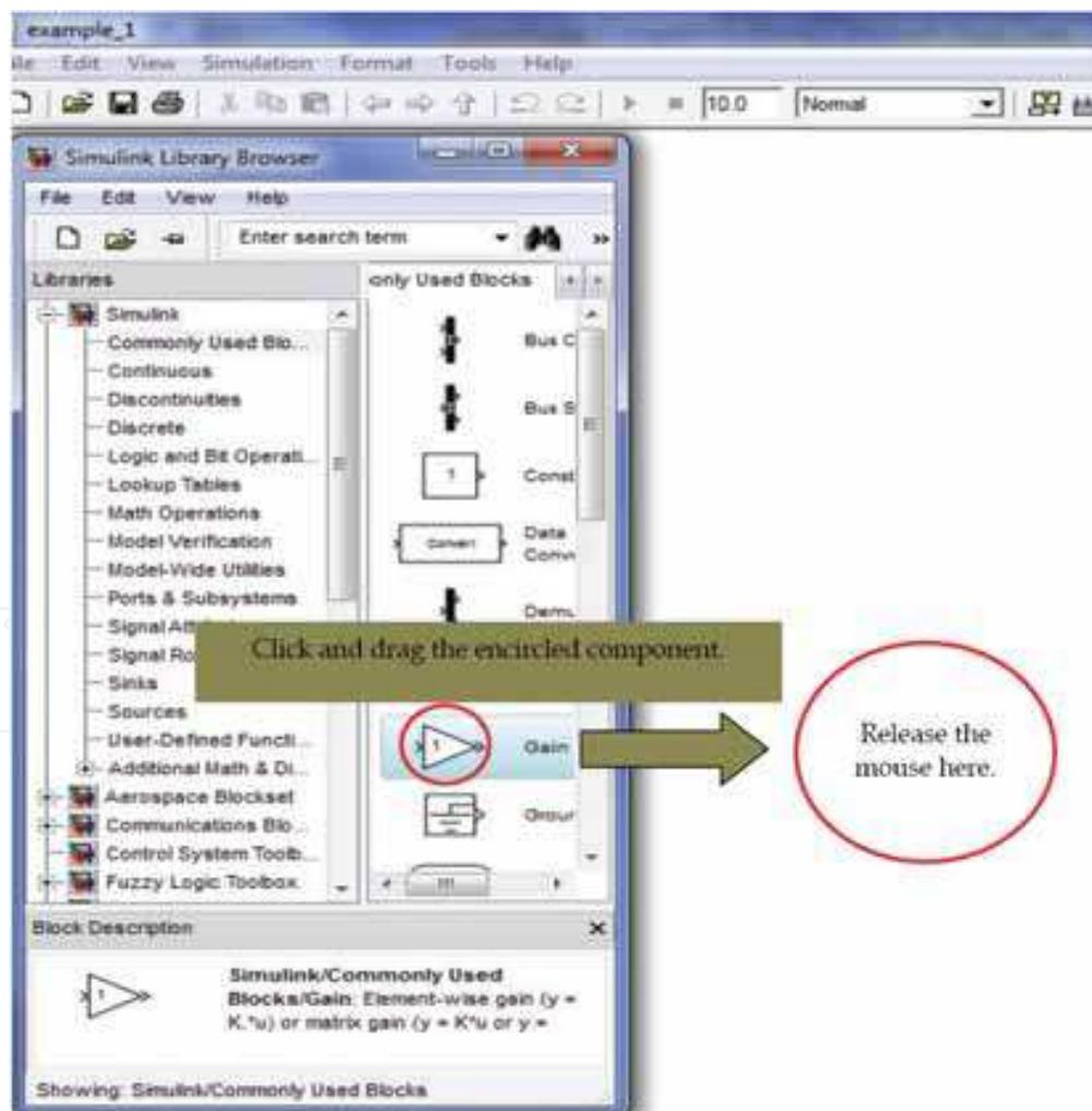
Fig. 7. Inserting blocks in a SIMULINK model
