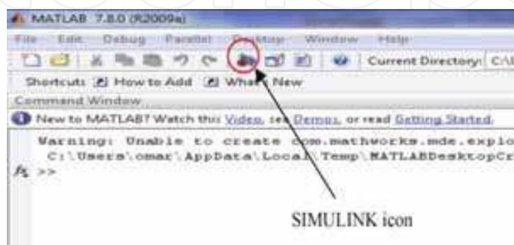
Fig. 3. Opening SIMULINK
