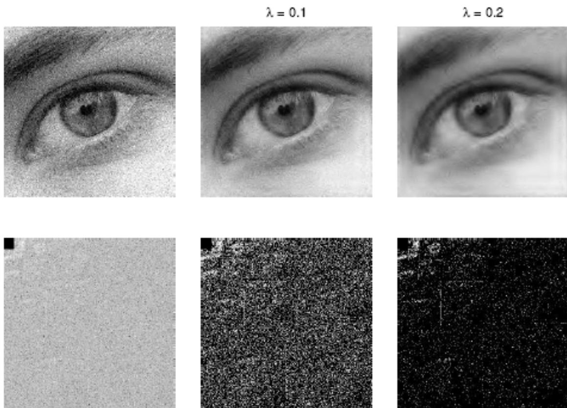
Fig. 3. Illustration of discrete wavelet shrinkage. The wavelet used here is the coiflet. Top row, from left right: the noisy image, wavelet shrinkage for different values of  $\lambda$ . The second row shows the discrete wavelet transform of the upper row.
