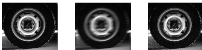
Fig. 5. RBFNN method result for Tire . True image(left); blurred image (middle); restored image(right), BSNR=11.22, ISNR=23.14
