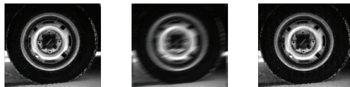
Fig. 9. Result for Tire . True image(left); blurred image (middle); restored image(right), BSNR=11.56, ISNR=22.09
