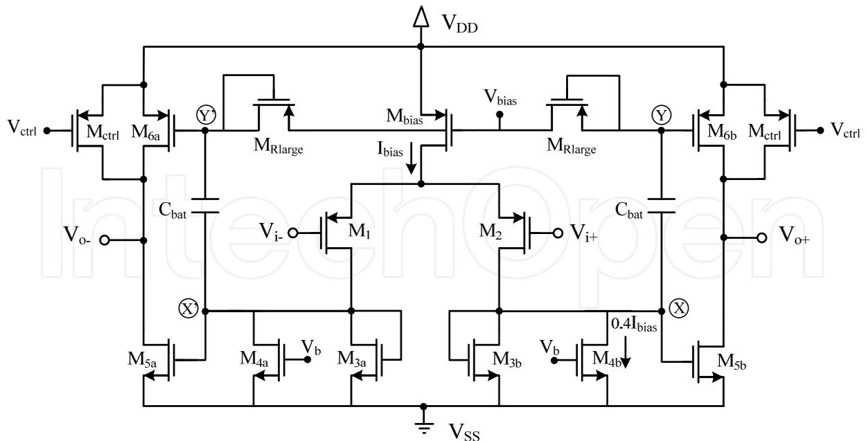
Fig. 4. Fully differential single-stage amplifier with class-AB output.
