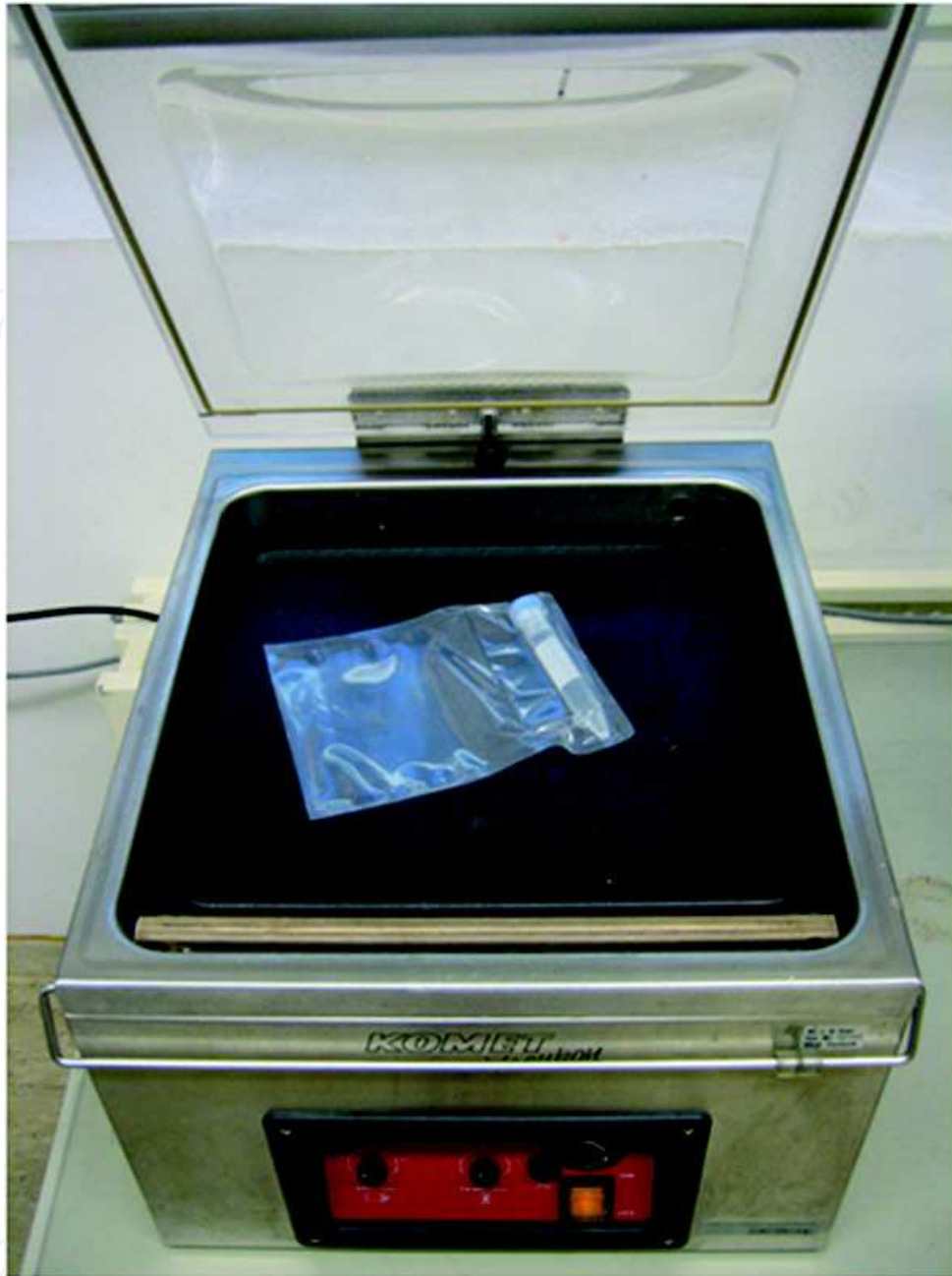
Fig. 2. Vacuum sealing device (Komet, Plochingen, Germany).
