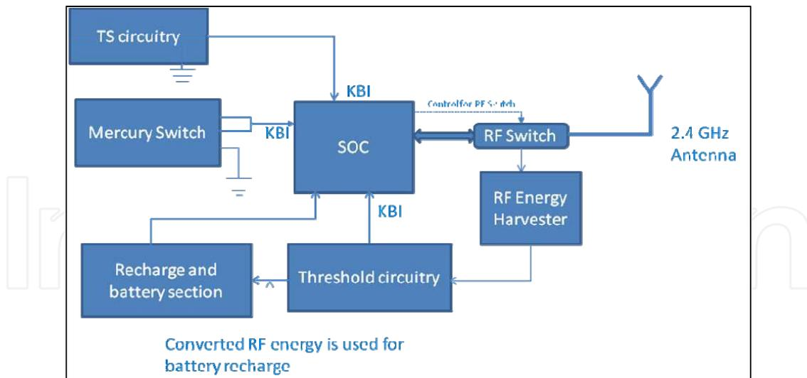
Fig. 1. Functional Block Diagram of the Sensor Node developed for Forest Monitoring
