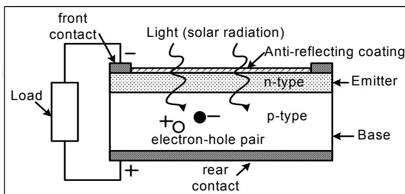
Fig. 5. General Structure of a Solar cell
