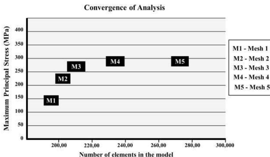
Fig. 7. Maximum principal stress ( $\sigma_{\max}$ ) in hypothetical convergence testing of mandible FE models meshed by 0.6 mm elements with no refinement (mesh 1) and with refinement levels 2, 3, 4 and 5 at a posterior implant region (meshes 2, 3, 4 and 5, respectively).
