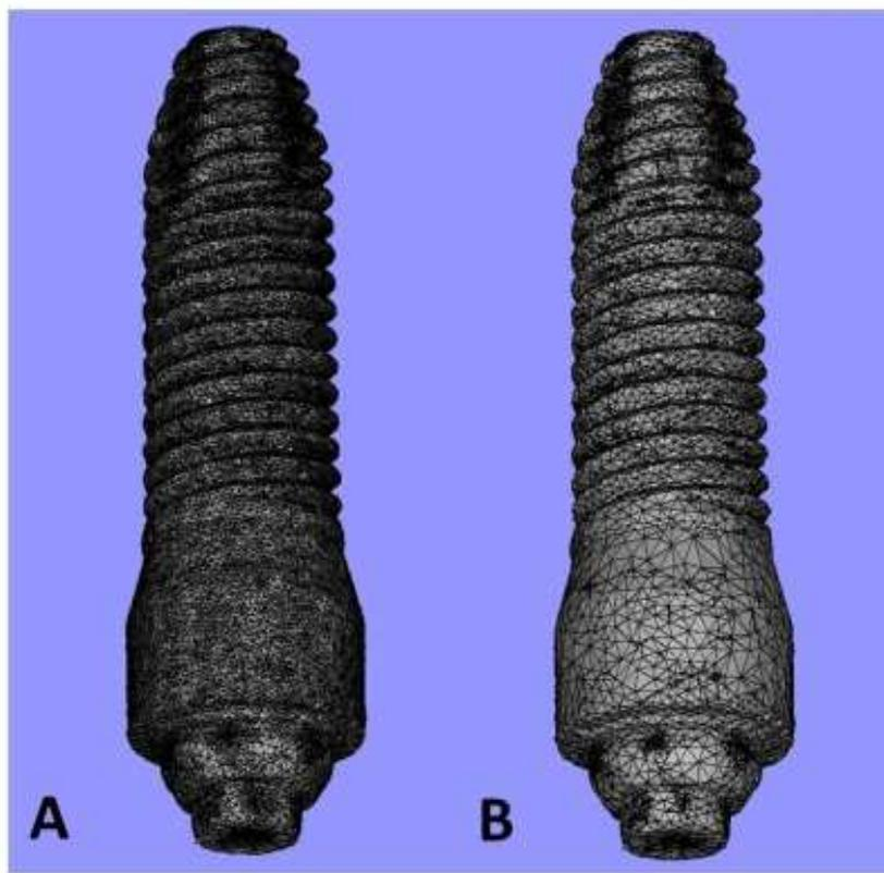
Fig. 3. (A) 3D CAD of the Nobel Speed™ RP Implant (Nobel Biocare, CA, USA) based on the micro-CT ( $\mu$ CT; CT40, Scanco Medical, Bassersdorf, Switzerland). (B) The Mimics Remesh (Materialise) function “quality preserving reduce triangle” and “reduce triangles” were used to reduce the number of elements at the implant CAD.
