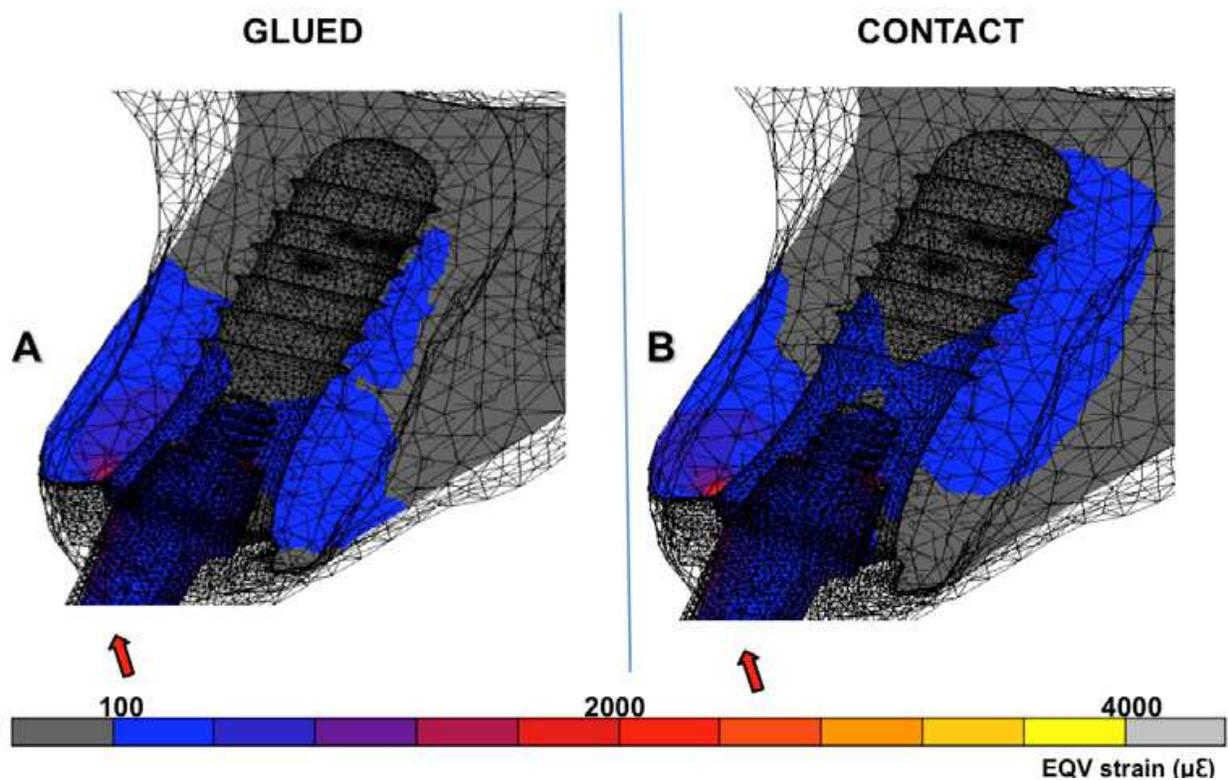
Fig. 5. Equivalent strain ( $\mu\epsilon$ ) distribution for 100N loaded implant in a superior central incisor region, in a median buccopalatal plane. The bone to implant interfaces were assumed as fixed bond ("glued") (A) and frictional contact (B). The arrows indicate the loading direction for clarity.
