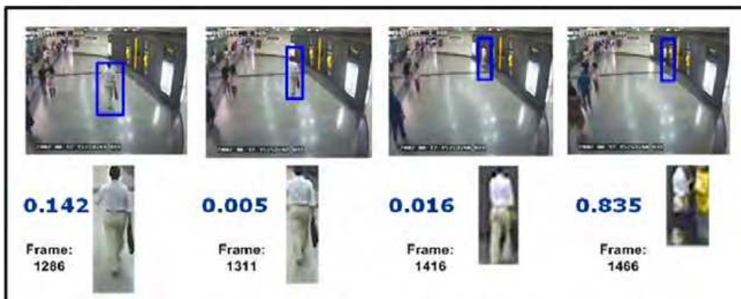
Fig. 9. An example of representative blob detection: 4 representative blobs are extracted from 905 blobs.
