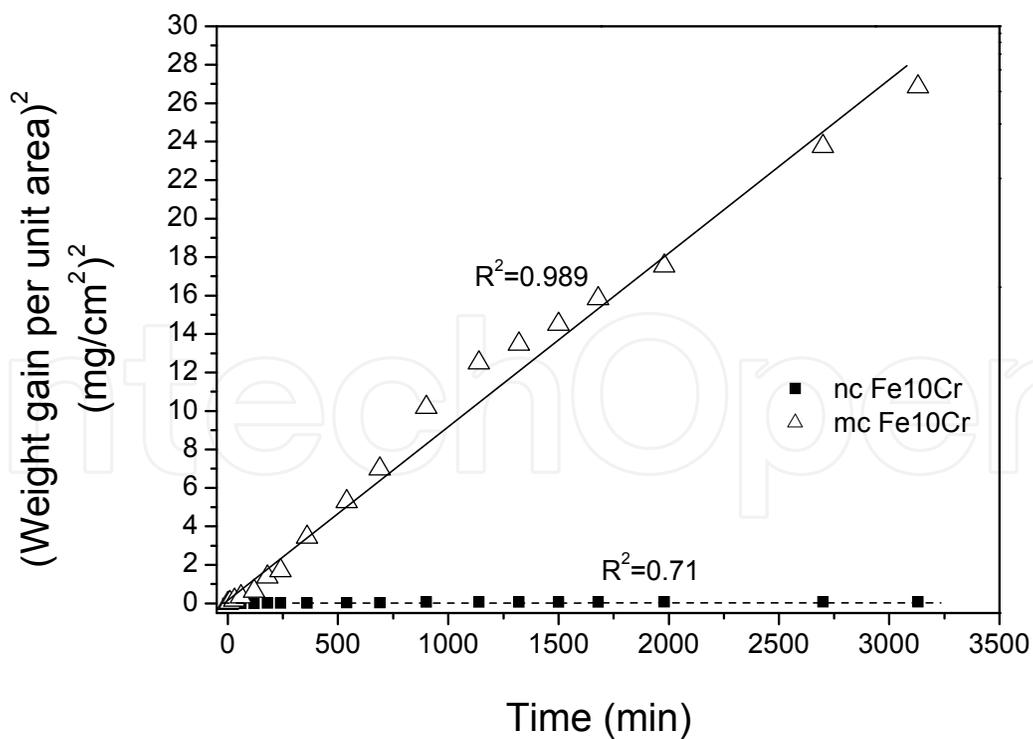
Fig. 6c. Oxidation kinetics of nanocrystalline (nc) and microcrystalline (mc) Fe-10Cr alloys, oxidised at 350°C: weight-gain<sup>2</sup> with time, suggesting parabolic kinetics for mc alloy but departure from parabolic kinetics for nc alloy [12,39].
