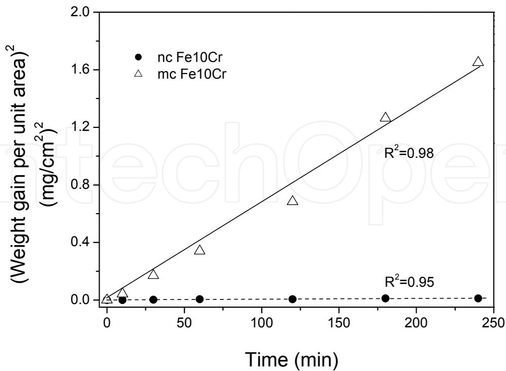
Fig. 6b. Oxidation kinetics of nanocrystalline (nc) and microcrystalline (mc) Fe-10Cr alloys oxidised at 350°C: weight-gain<sup>2</sup> with time (up to 240 minutes) suggesting parabolic kinetics for both mc and nc alloys [12,39]
