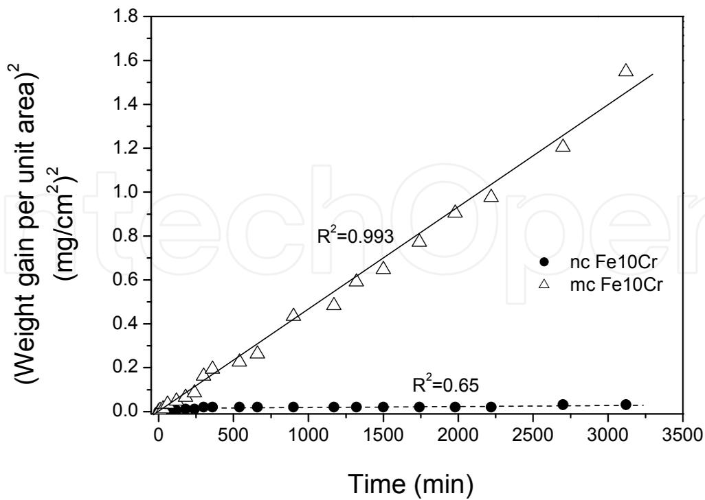
Fig. 5c. Oxidation kinetics of nanocrystalline (nc) and microcrystalline (mc) Fe-10Cr alloys, oxidised at 300°C: weight-gain<sup>2</sup> with time, suggesting parabolic kinetics for mc alloy but departure from parabolic kinetics for nc alloy [12,37,39].
