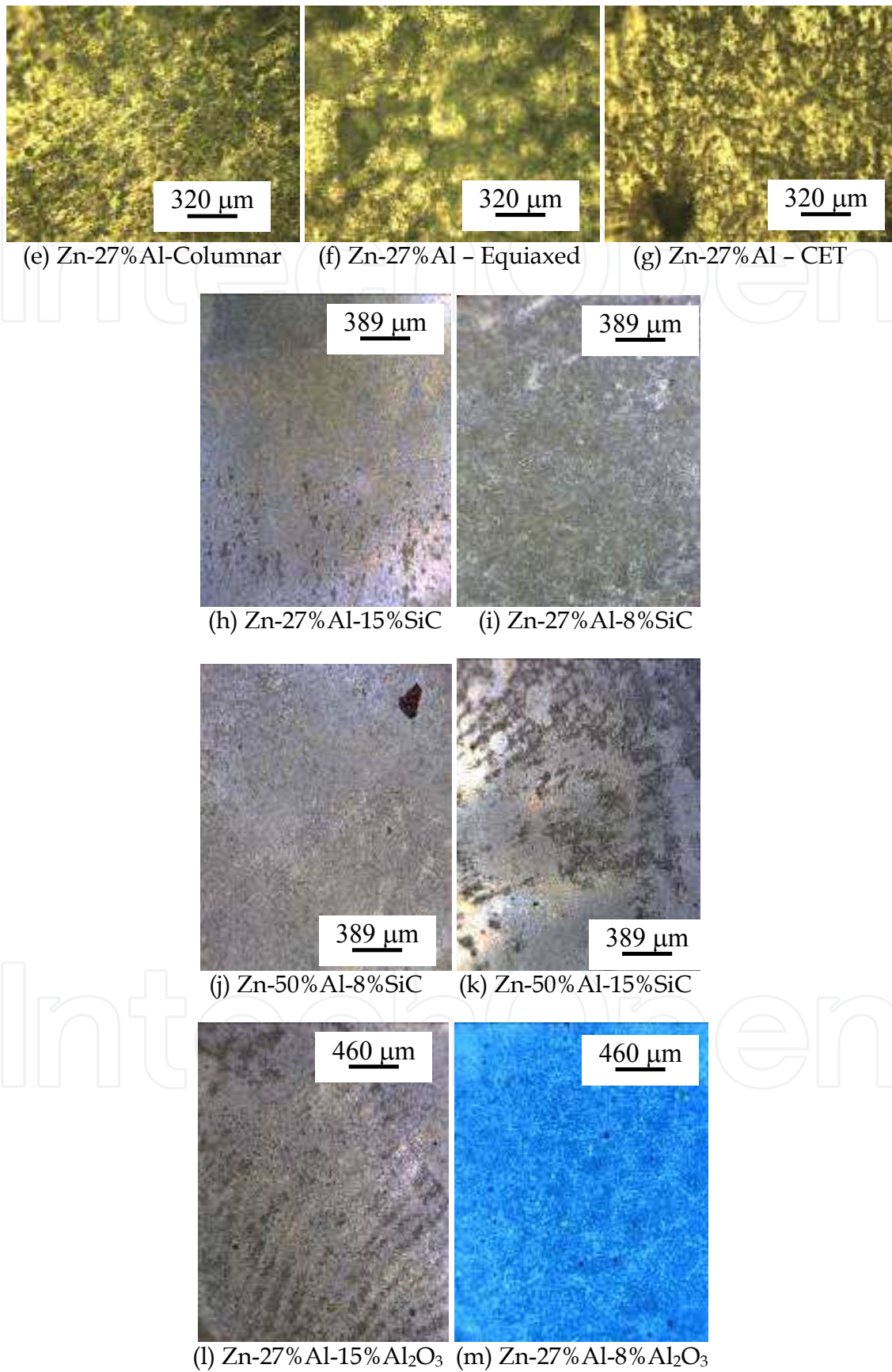
Fig. 3. Micrographs of different alloy samples and structures.
