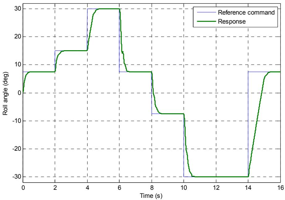
Fig. 9. Roll-angle-tracking performance at high speed (30km/h)
