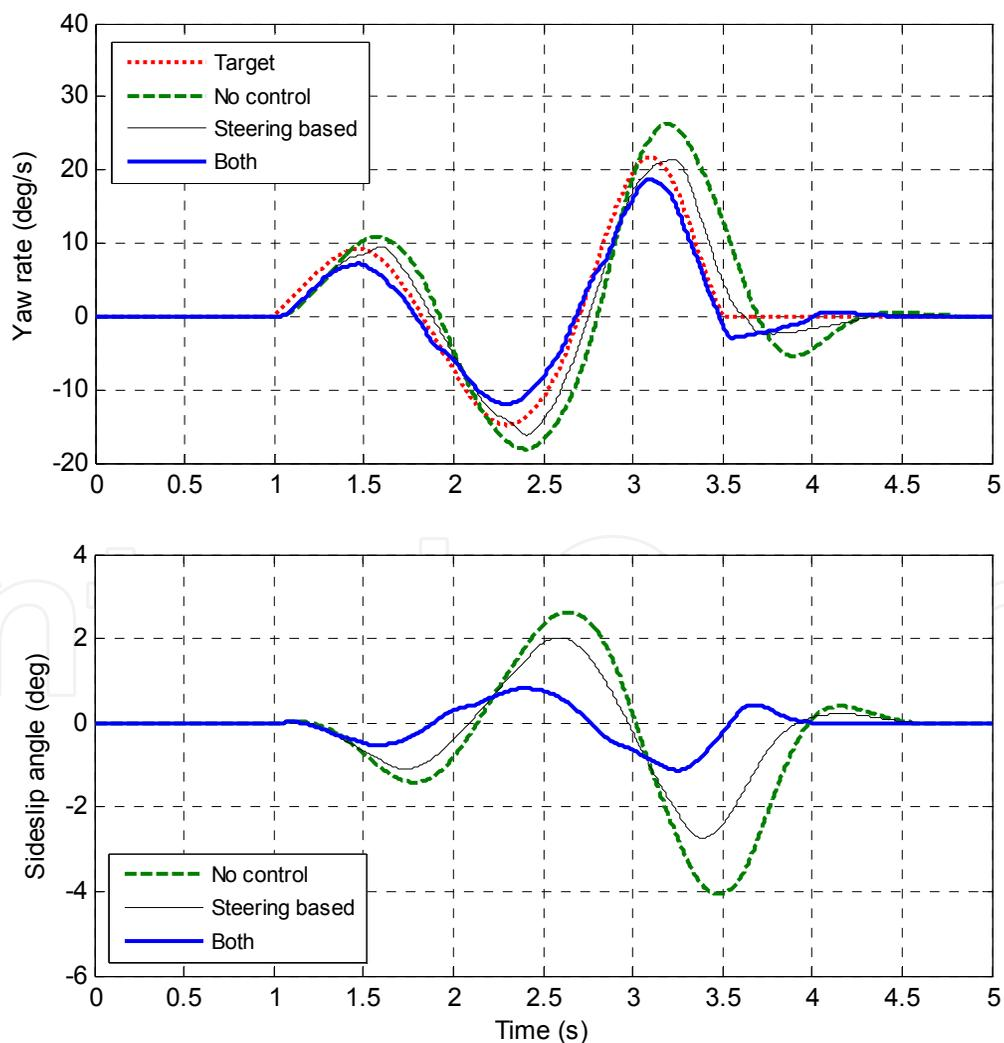
Fig. 16. High friction:  $\mu = 0.85$ ; normal speed:  $V_x = 100\text{km/h}$
