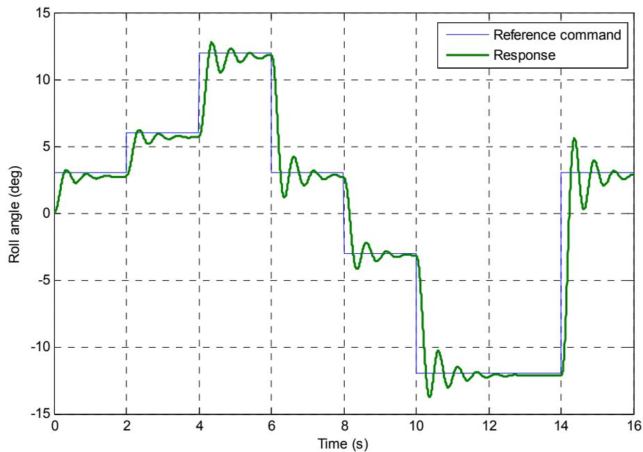
Fig. 6. PID controller performance at normal speed (12km/h)
