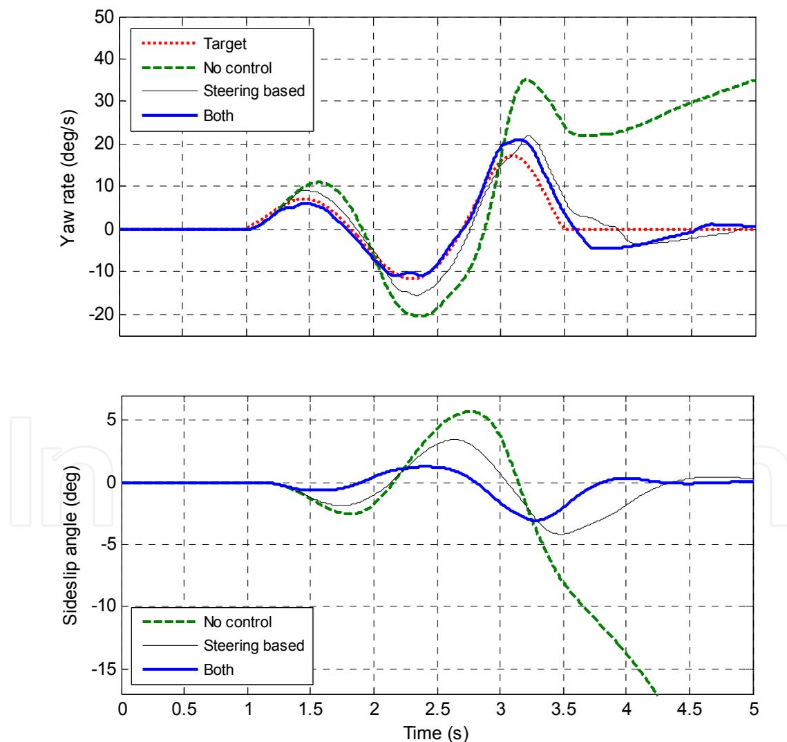
Fig. 17. High friction:  $\mu = 0.85$ ; high speed:  $V_x = 180\text{km/h}$
