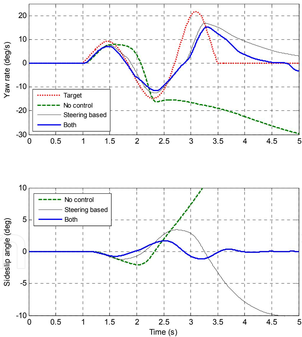
Fig. 19. Low friction:  $\mu = 0.2$ ; normal speed:  $V_x = 100\text{km/h}$
