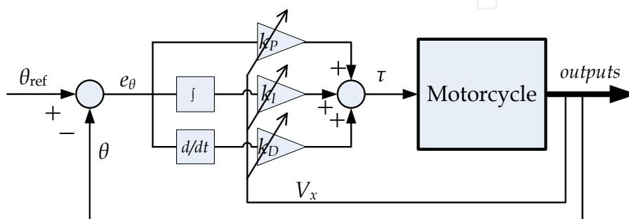
Fig. 4. Roll-angle-tracking controller for motorcycle (Sharp et al., 2005)
