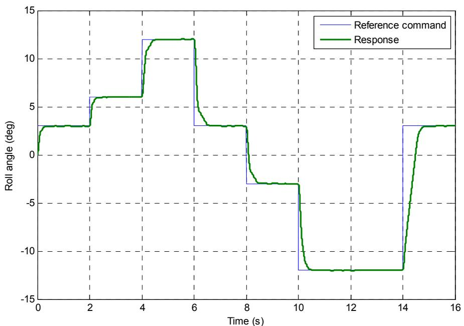
Fig. 7. Roll-angle-tracking performance at low speed (5km/h)
