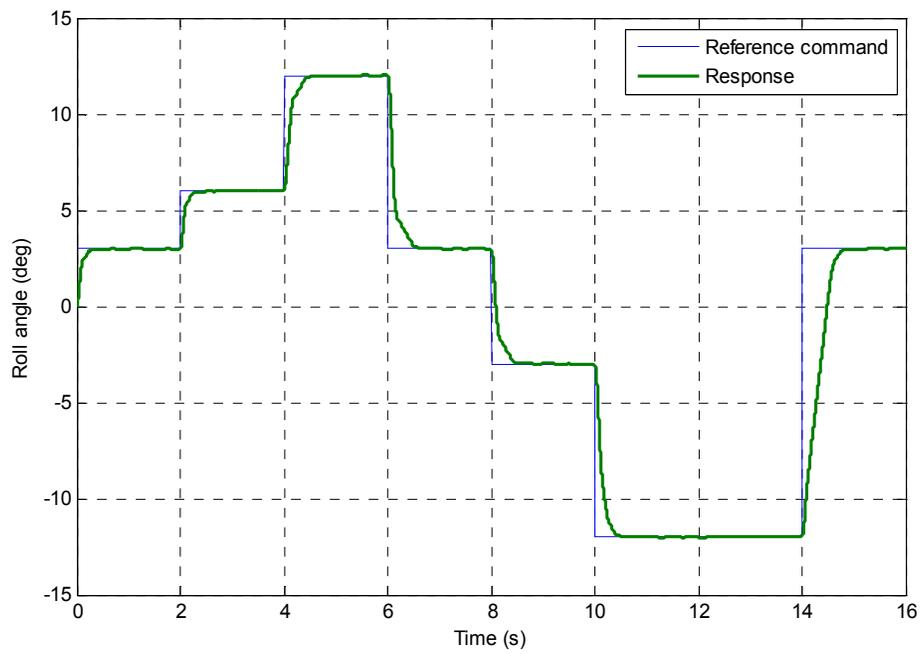
Fig. 8. Roll-angle-tracking performance at normal speed (12km/h)
