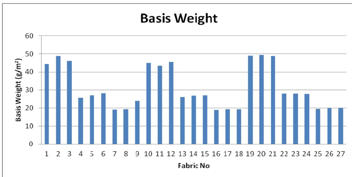
Fig. 2. Basis weight values of polypropylene meltblown nonwovens
