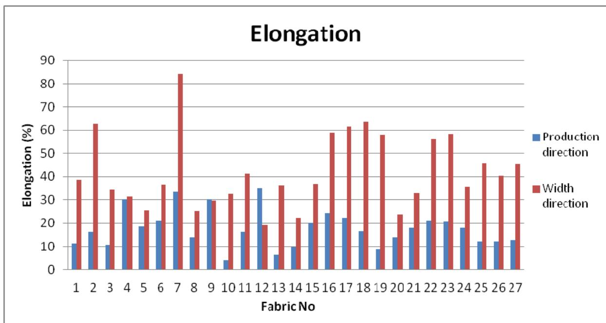
Fig. 6. Elongation values of polypropylene meltblown nonwovens
