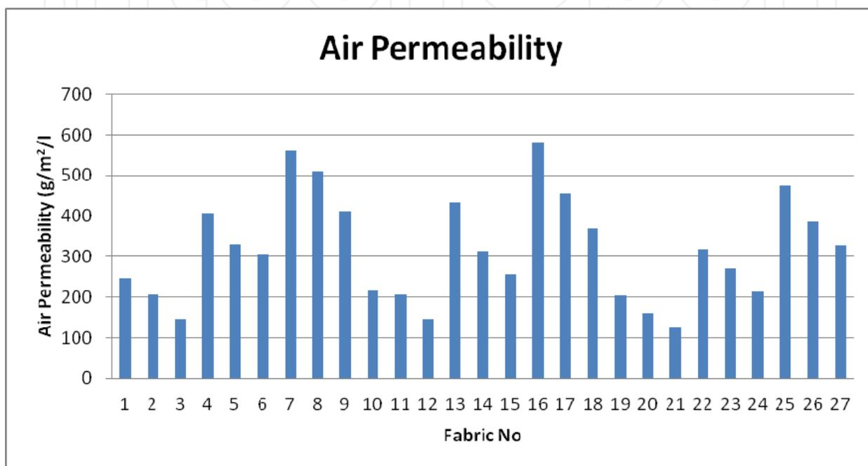
Fig. 3. Air permeability values of polypropylene meltblown nonwovens
