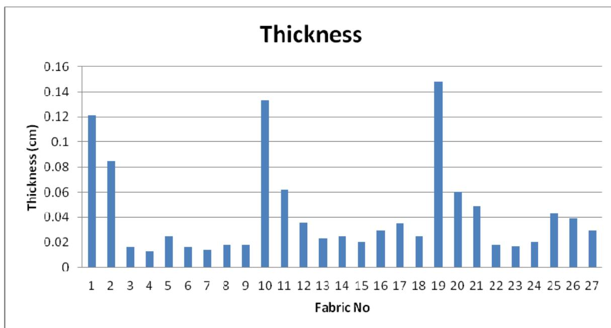
Fig. 1. Thickness values of polypropylene meltblown nonwovens
