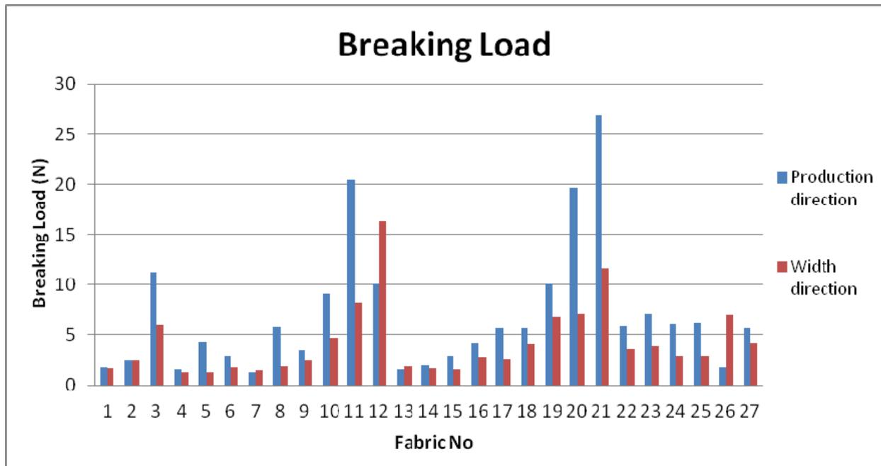
Fig. 5. Breaking load values of polypropylene meltblown nonwovens
