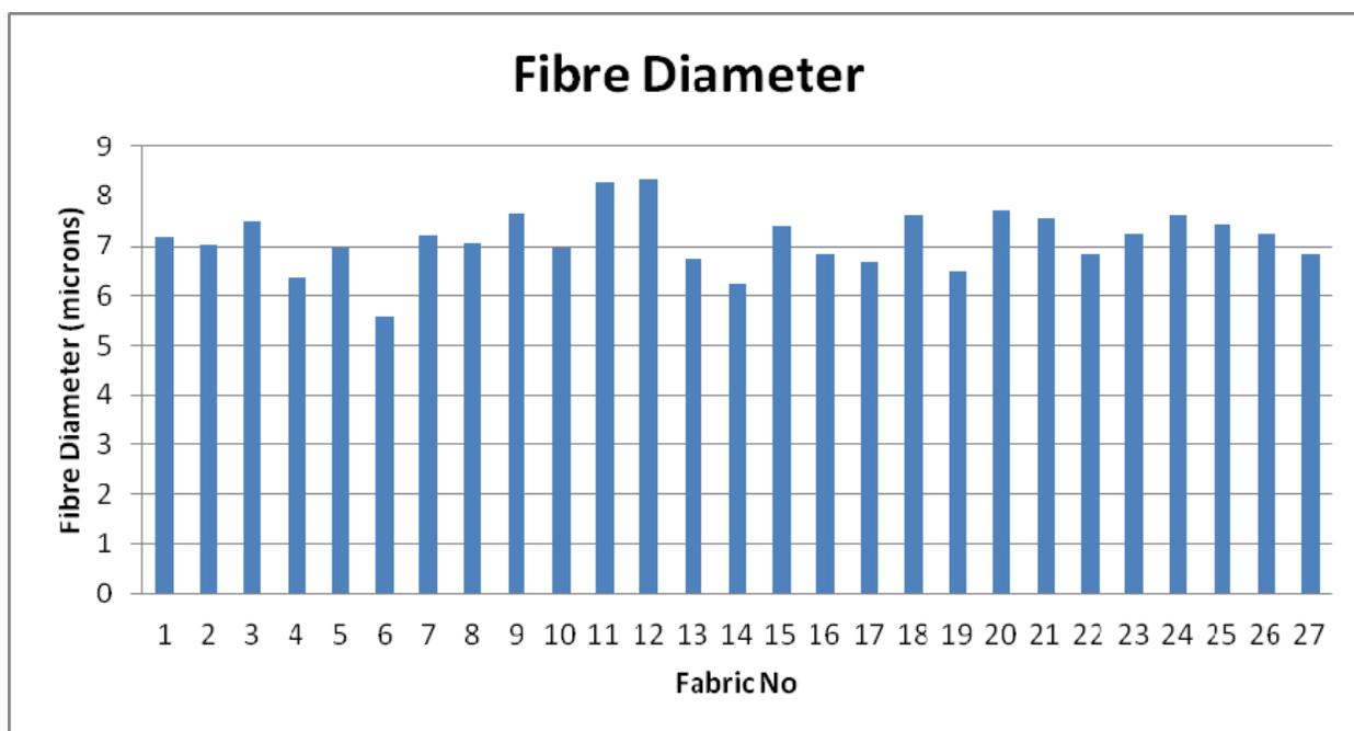
Fig. 4. Fibre diameter values of polypropylene meltblown nonwovens
